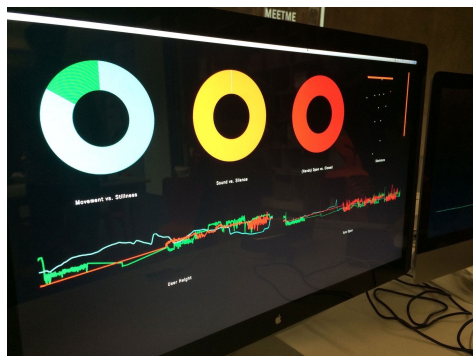
Figure 25 Initial experiments showing live information graphs of sensor data using the D3 web framework (Figure 22 Above)
