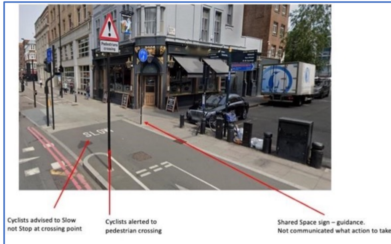
Figure 4.43 Shared Space artefacts installed
