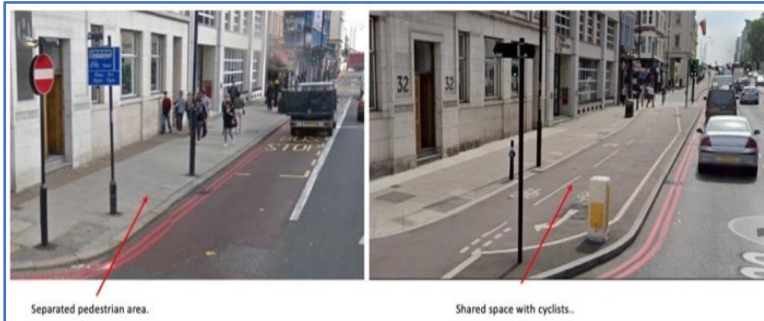
Figure 4.44 Disaffordance - removal of pedestrian space to cross the road
