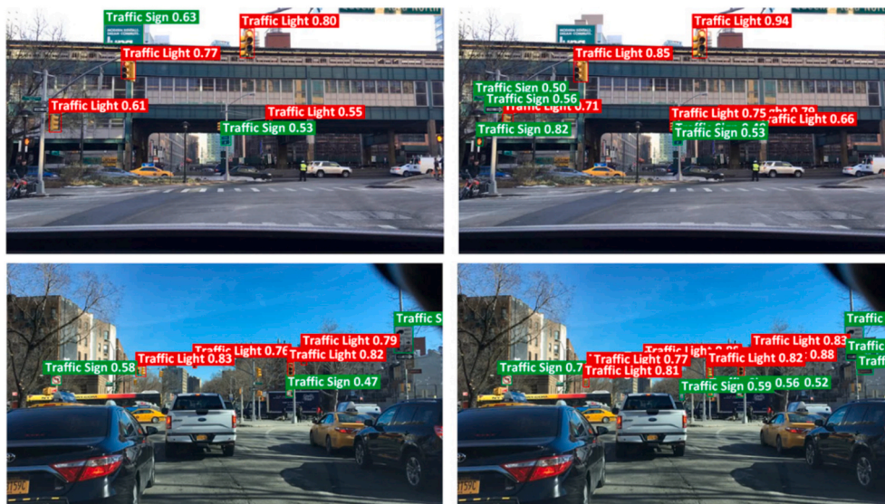
Fig. 2. Detection performance comparison in varying traffic environments: (a) YOLOv5 and (b) improved Scaled (iS)-YOLOv5. As traffic density increases from top to bottom, YOLOv5's prediction confidence decreases, leading to missed targets. In contrast, the proposed iS-YOLOv5 model maintains high confidence in detecting traffic signs and traffic lights, even in high-density traffic scenarios. This figure is regenerated from Fig. 8 of reference ( Mahaur and Mishra, 2023 ).
