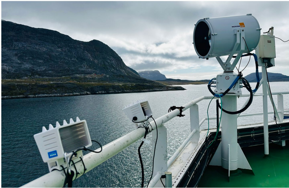
Figure 5. GoPro and Insta Ace Pro Cameras installed in shrouds designed by the research team on the rail over the wheelhouse top bridge wings on the James Cook approx. 25 m above sea level. Set to a transect timing ever 3 s (based on an average ship's cruising speed of 10 knots providing image overlap) 24 h a day in the EZ (international waters).
