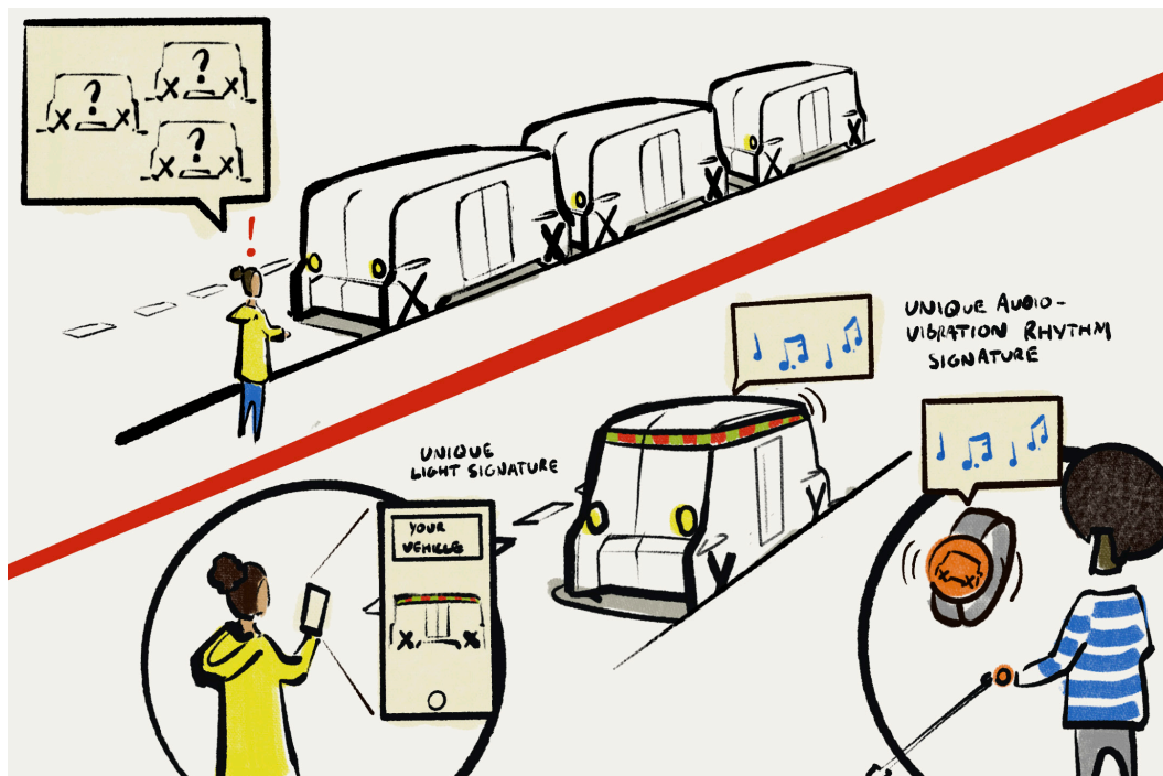
Storyboard sketches showing audio, visual, and haptic means of vehicle identification using smartphone apps and SAV-specific wearable device
