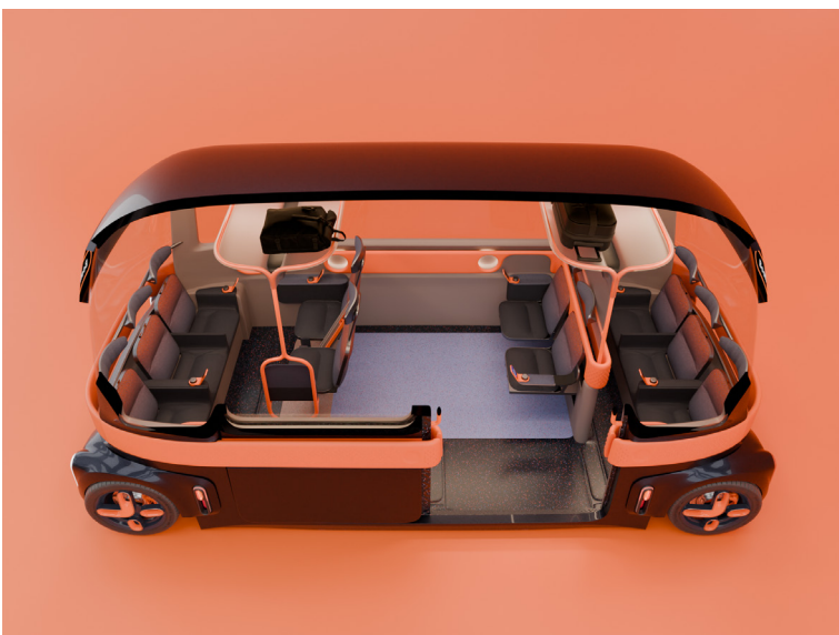
SAV layout maximising forward-facing seating.
