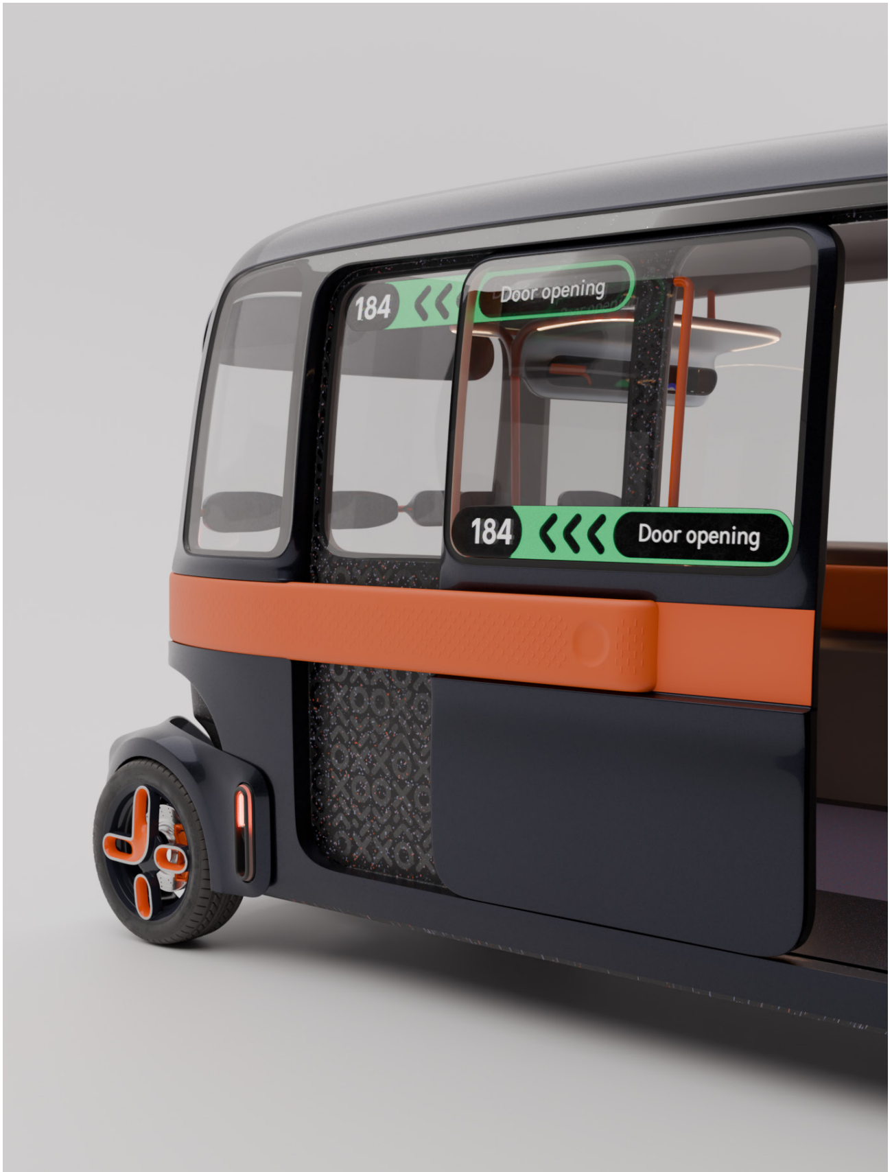
SAV exterior with side eHMI showing door opening indicators.
