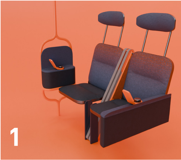
Reversible seat design shown in 3 positions.
