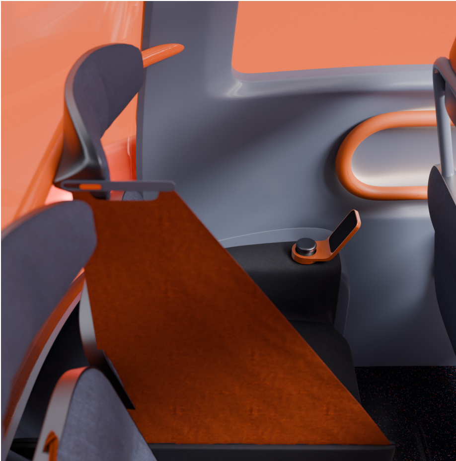
Retractable textile divider between seats at front and rear of vehicle.
