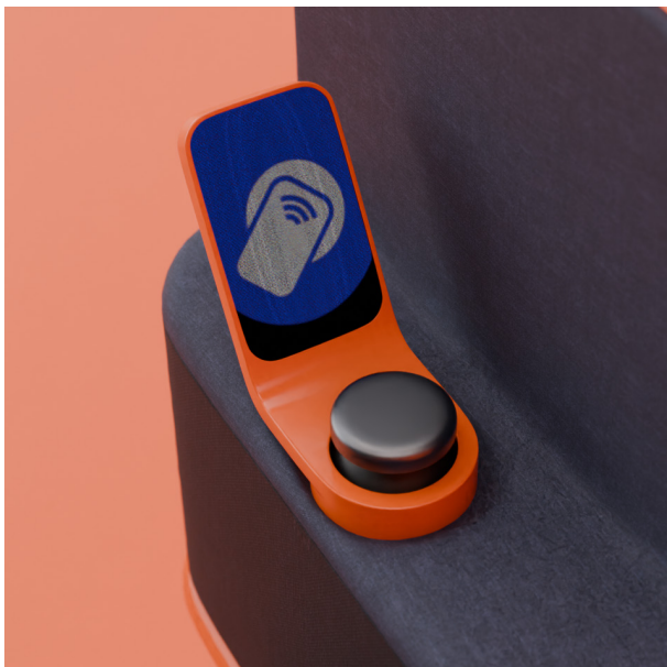
At-seat interface with travelcard icon prompting passengers to tap their card to show specific journey details etc.
