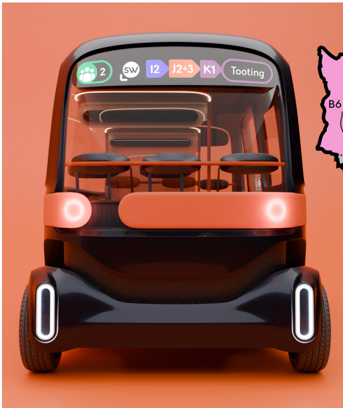
eHMI design for hailing with availability, direction, zones, and destination shown
