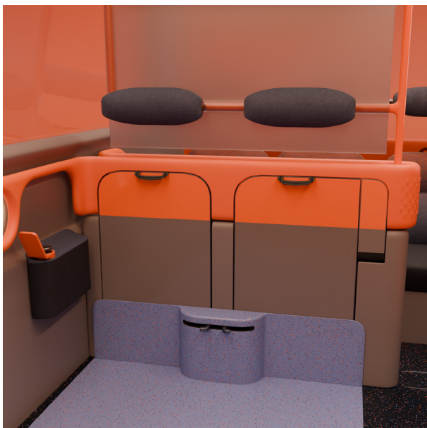
Wheelchair space folding seating in folded and unfolded positions
