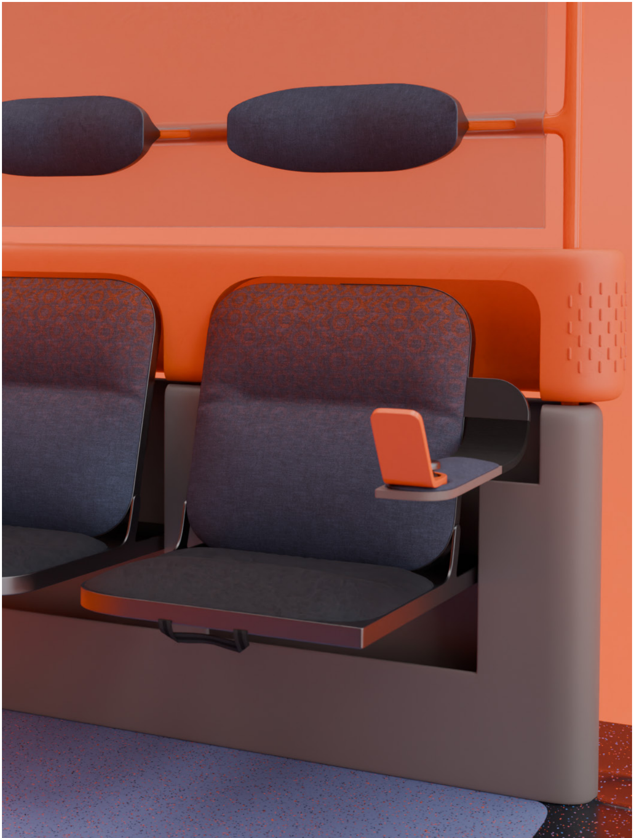
At-seat interface location for fixed folding seat. Interface attached to folding armrest.
