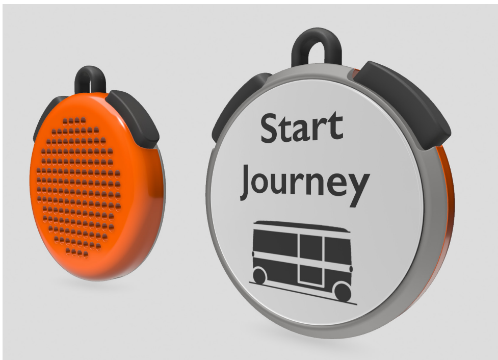
Concept SAV-specific device with simple button-based interactions, e-paper display and audio output.
