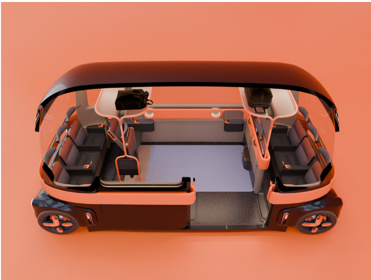
SAV layout for wheelchair user facing a travelling companion in a reversible seat.
