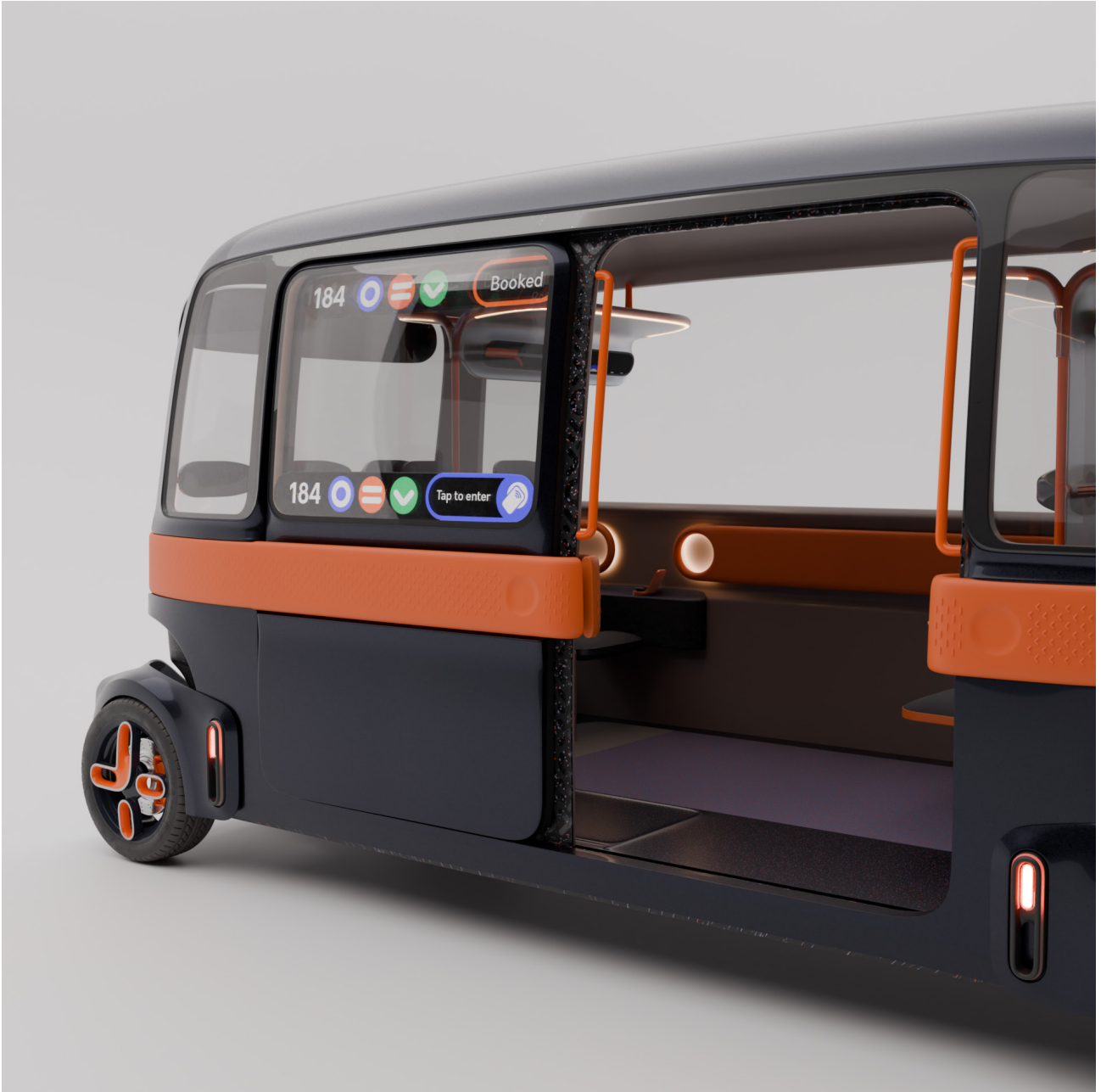
Vehicle exterior showing handles and guide rails.
