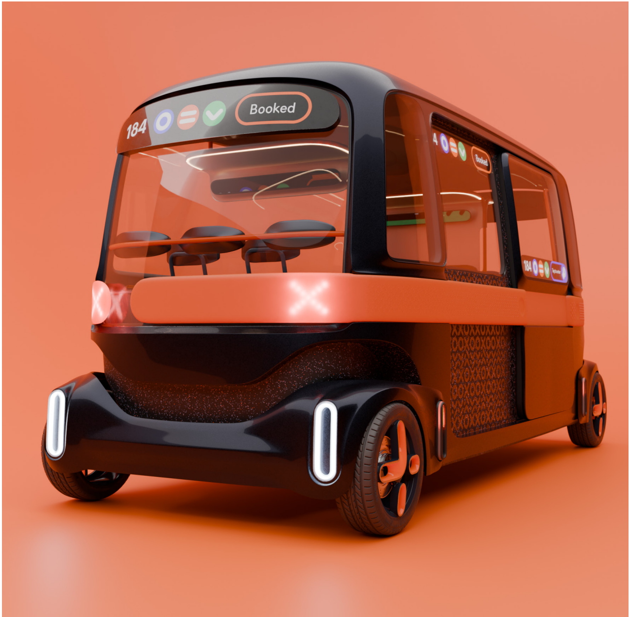
SAV exterior with front eHMI showing simple number, colour, and symbol based means of identification.
