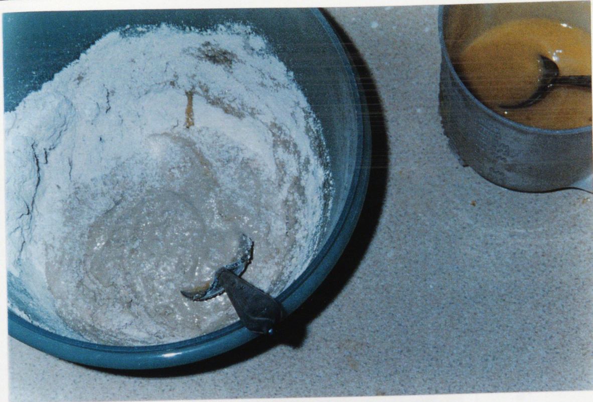
Fig. 137 Adding the compo "juice" to the sifted whiting.
