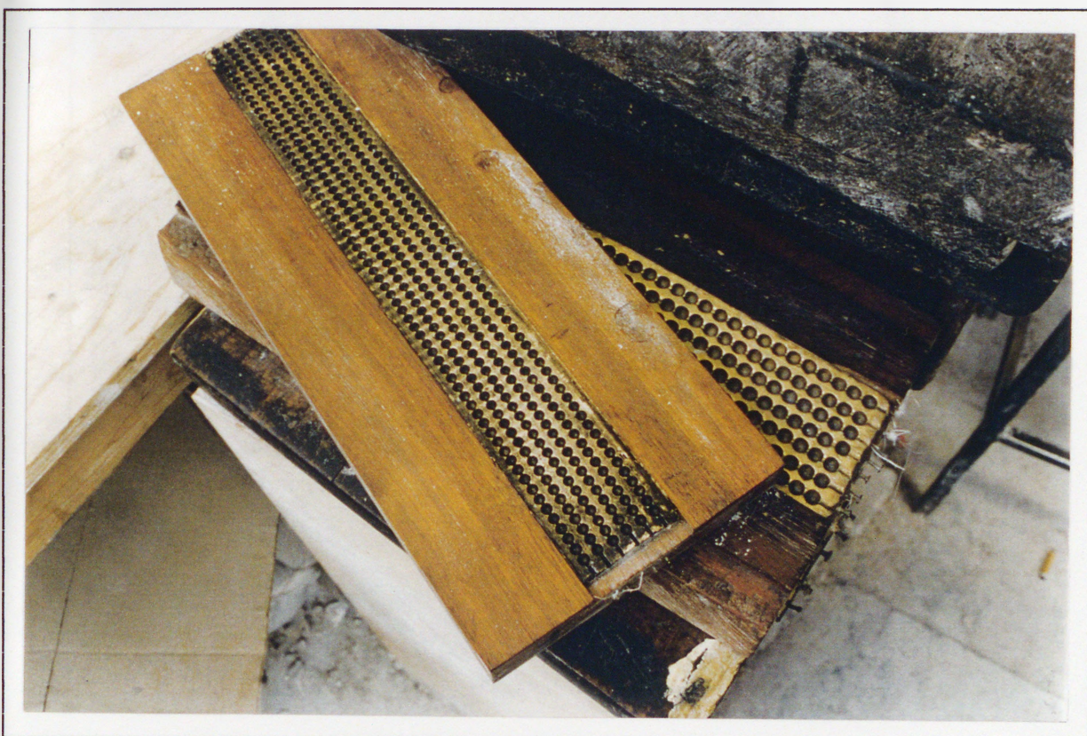
Fig. 10 Brass moulds for pearl beading (Collection of George Jackson & Sons). The threads to keep the lines together are hooked tight over the pins in the ends of the blocks before compo is applied.
