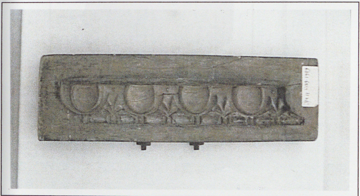
Fig. 49 A mould that has split along its grain and has been bolted together, Jackson Collection, Victoria & Albert Museum.
