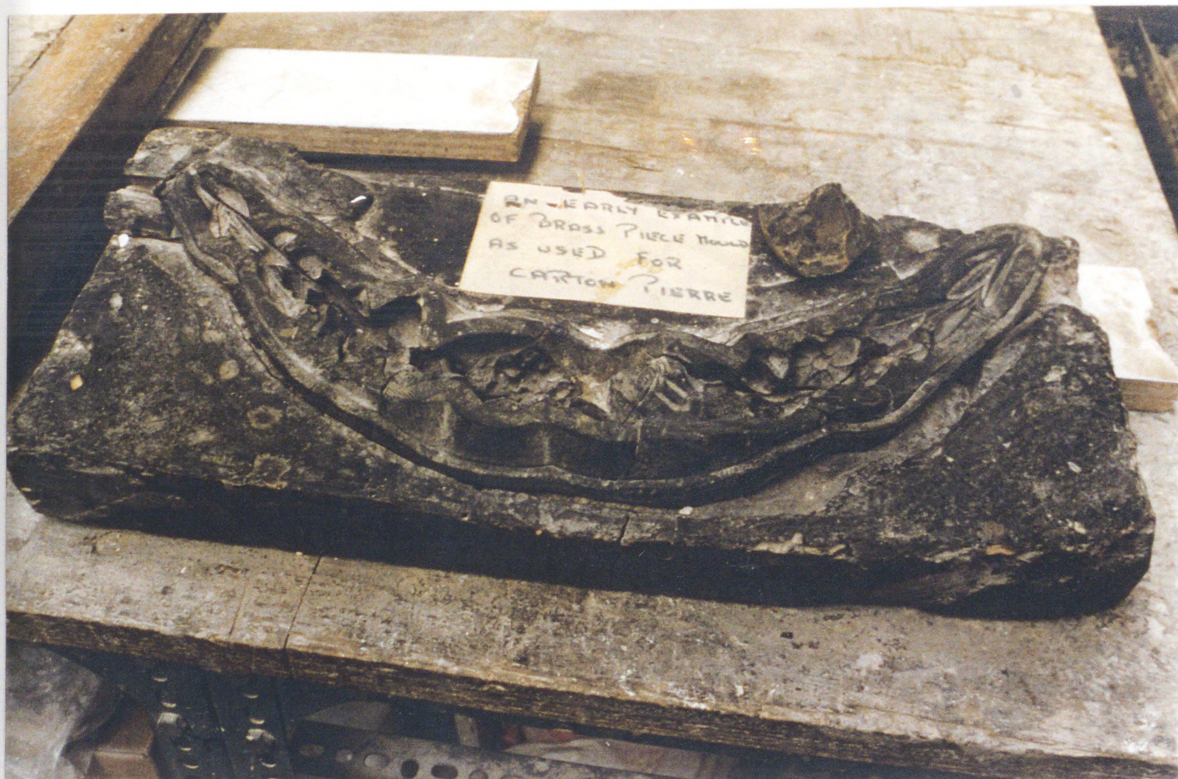
Fig. 12 Brass piece-mould for a flower swag (Collection of George Jackson & Sons).
