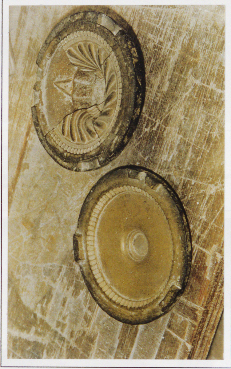
Fig. 16 Brass piece mould for the decoration round a candle drip tray on a girondole or candelabrum, (Collection of George Jackson & Sons).
