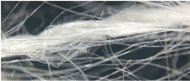
Image 5.1 Microscopy of mohair yarn Ariane Fourquier (2023)
