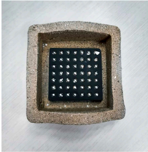
FIGURE 15 3 mm granules inside the custom saggar made from crank clay. Note the bright, polished appearance of the granules and slight cracking of the saggar after repeated use. Courtesy of Katharina Vones, 2023.
