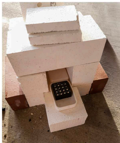
FIGURE 12 The cooling station assembled from loose firebricks. Courtesy of Katharina Vones, 2023.
