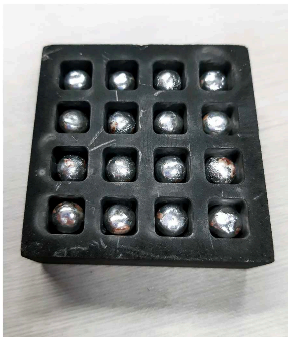
FIGURE 14 Granules of 6 mm inside the Graphite setter, straight out of the furnace. Note the bright, even surface of the granules. Courtesy of Katharina Vones, 2023.
