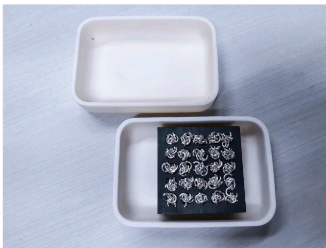
FIGURE 11 The 5 mm graphite setter fully loaded with Britannia silver jump rings inside the alumina crucible used during the first set of experiments. Note the difficulty in fitting the appropriate amount of silver into the divots. Courtesy of Katharina Vones, 2023.
