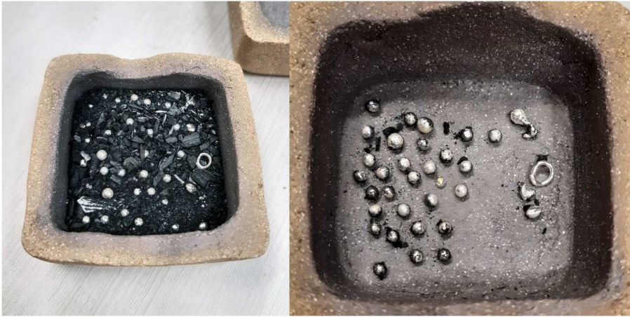
FIGURE 8 Experiments with the traditional charcoal layering technique undertaken as part of the Fire Arts Symposium. Note the variation in size of granules despite starting with wire jump rings of equal size, and partial melting of some fragments. Courtesy of Katharina Vones, 2023.
