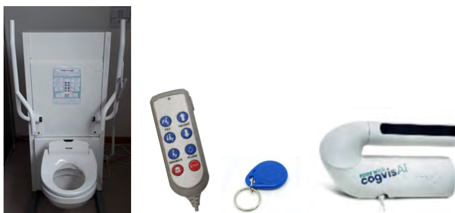
Figure 8. The final T4ME2 prototype 2 (PT2) with some of its main components: A wall-mounted ICT-enhanced motorised lift toilet (with shower seat add-on and built-in air quality sensor), an 8-buttons hand control, RFID tags (e.g. for recalling pre-stored individual settings) and a smart and privacy-aware 3D sensor for safety and presence detection. See (T4ME2 virtual room, 2022) for a clickable online demonstration of the PT2 and the whole toilet room
