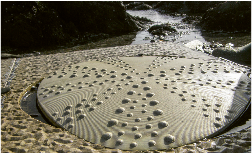
The Hannafore Outflow Pipe Project , test samples manufactured from concrete and attached to the surface of the pipe. Its intention to observe the human and ecological response to the designs over a five-month deployment trial. Credit | Daniel Metcalfe.
