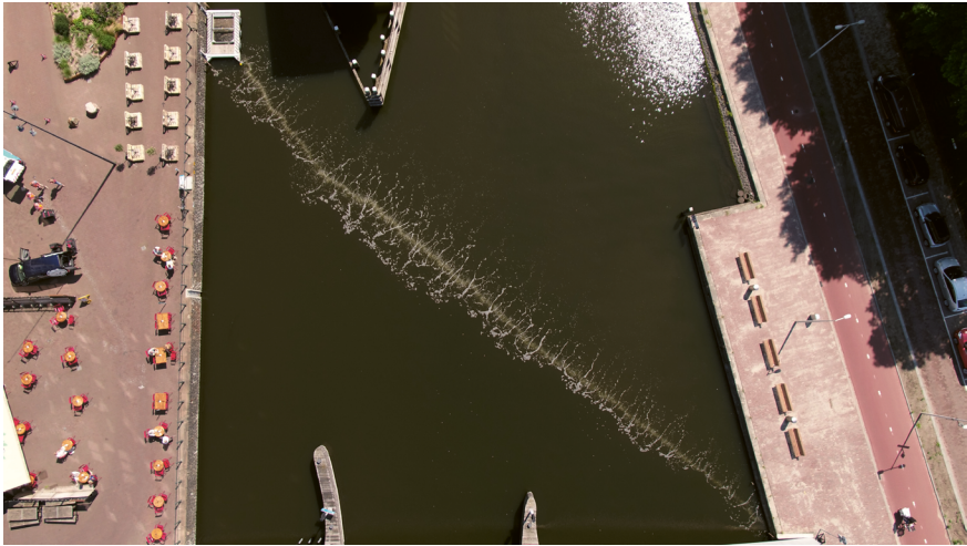
The Great Bubble Barrier is a semi-permanent cost-effective technology producing an air curtain, capturing detritus in rivers or estuaries, removing waste before it enters the sea. A drone photograph of deployment in Amsterdam. Credit | The Great Bubble Barrier.
