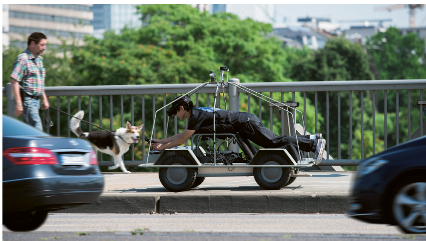
Who Wants to be a Self-driving Car? The unconventional driving machine lets people use real-time, three-dimensional mapping and object recognition, displayed in a virtual reality headset to navigate spaces. Credit | Joey Lee.
