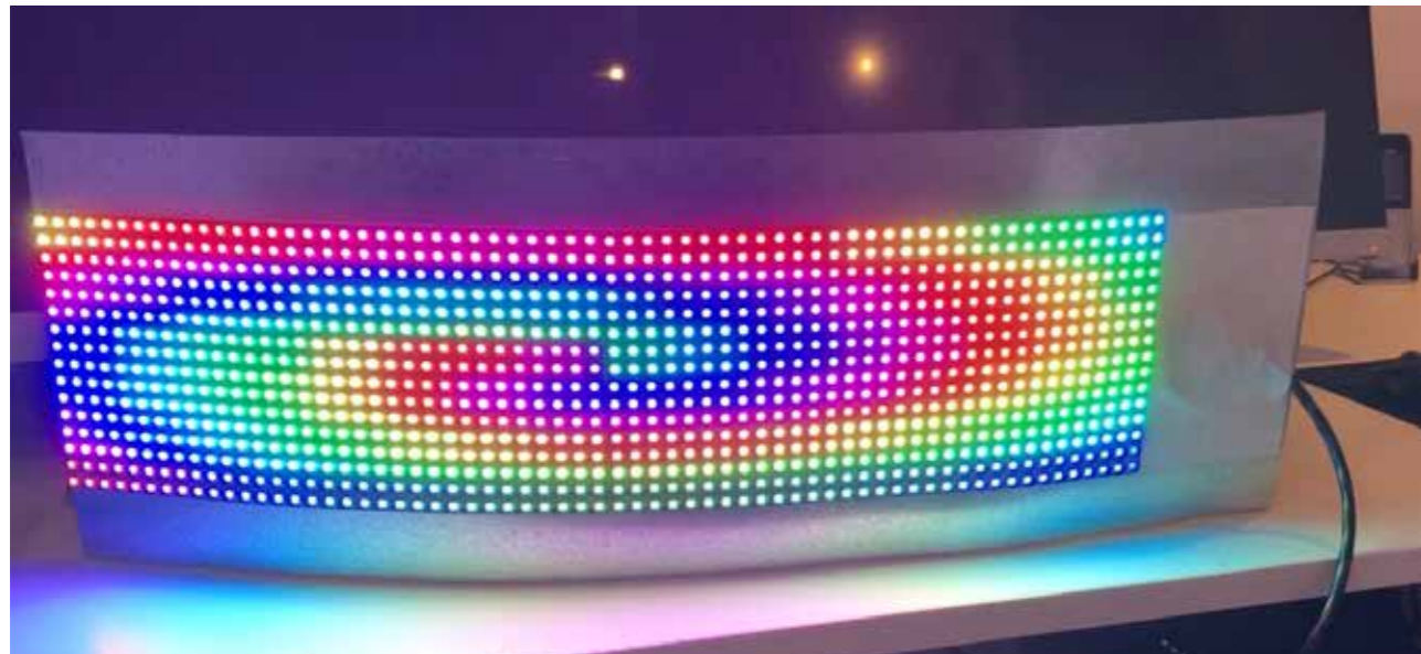
Figure 78: Photograph of the magnetic back digital communications unit on a curved galvanised steel backing plate. Test colour display.
