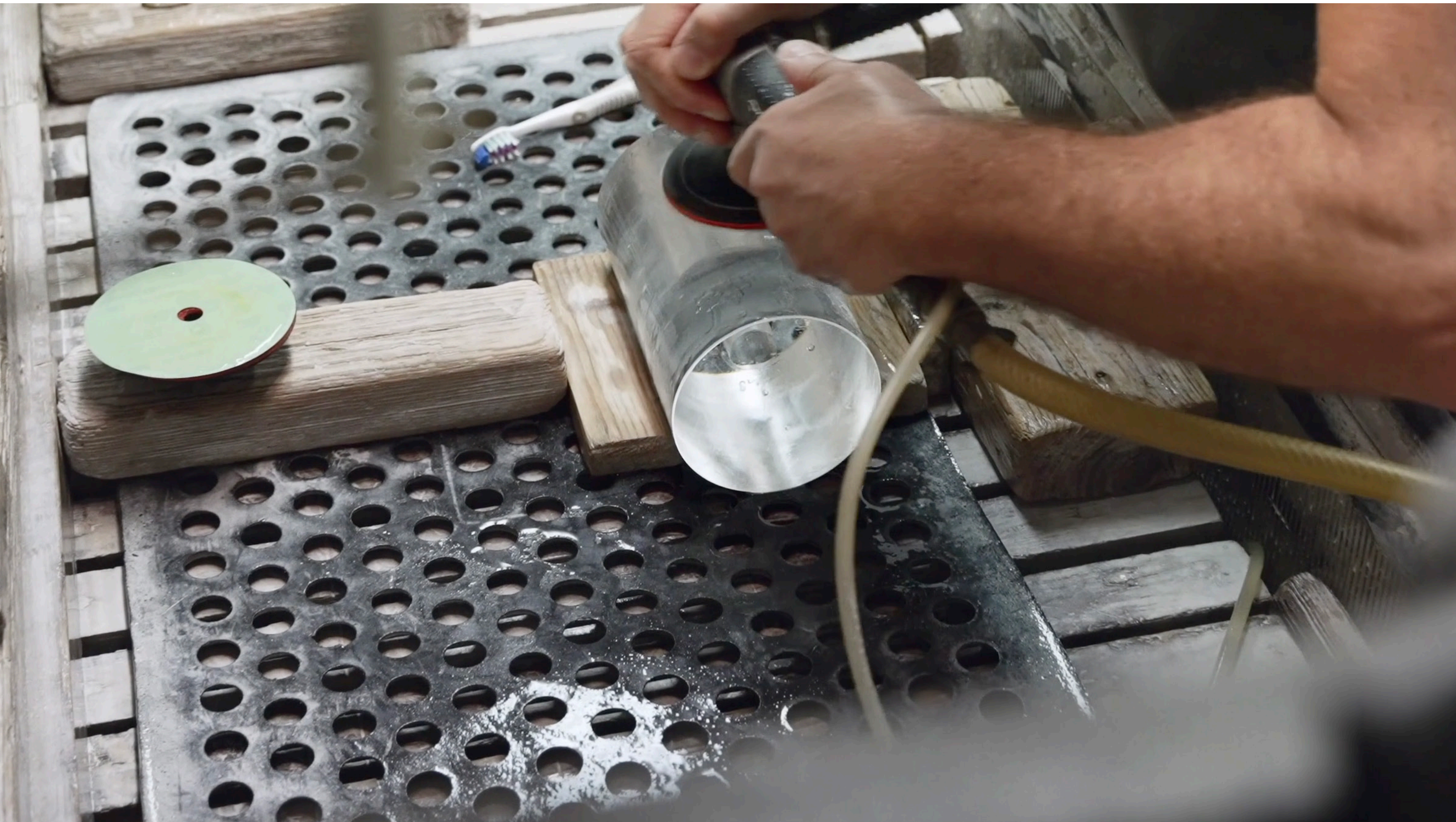
Fig.32 '1765 - Antarctic Air' production still from Polar Zero documentary film. Polishing cast glass
