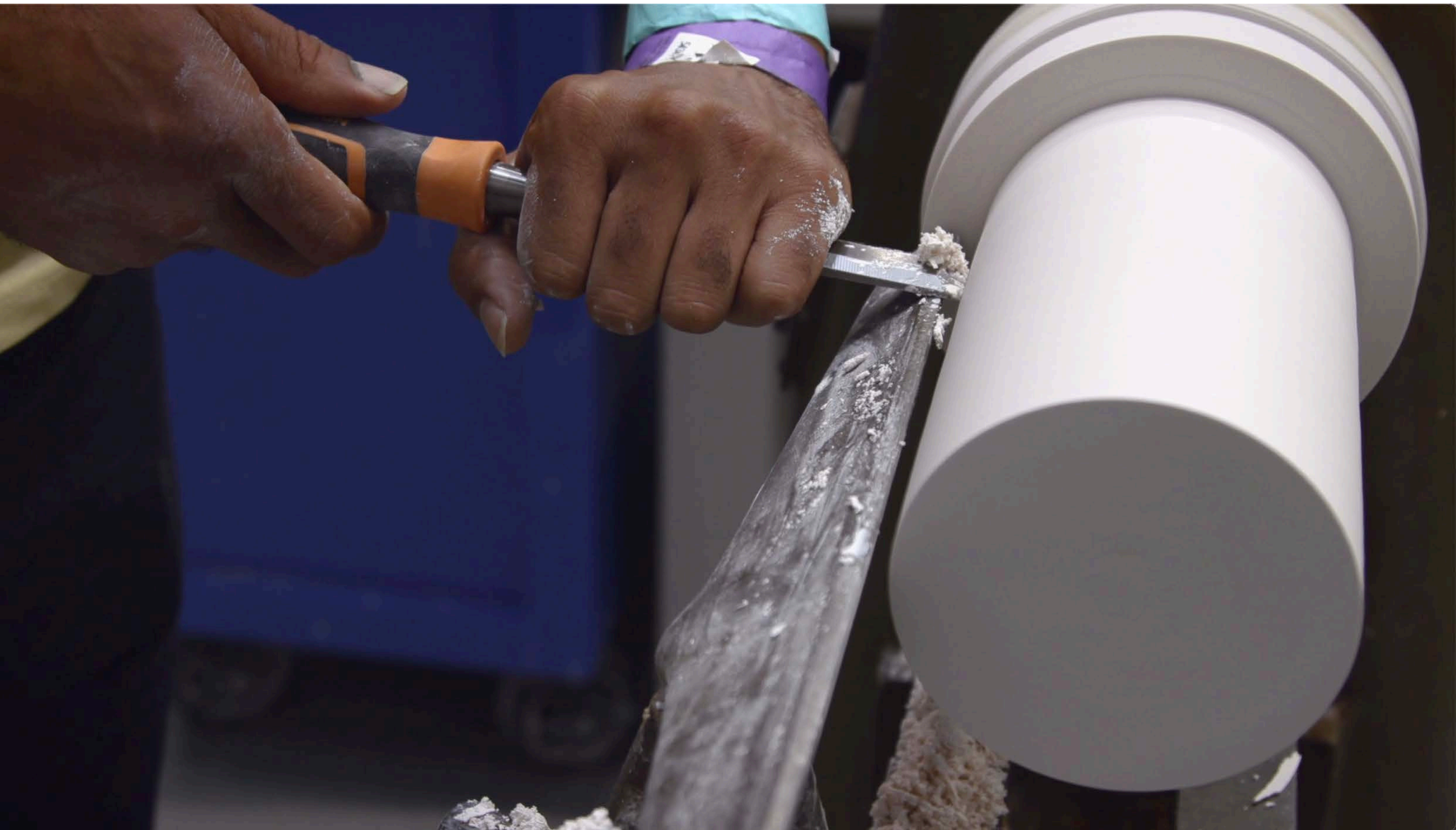
Fig.29 '1765 - Antarctic Air' production still from Polar Zero documentary film. Lathe working the plaster model for glass casting. RCA
