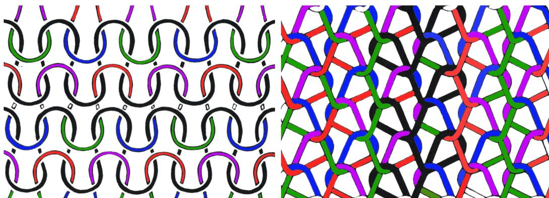
Figure 5.4 Weft knitted structure coloured with TA mapping
