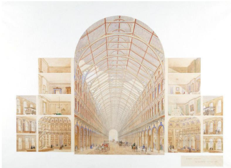
Fig. 97: Cross-section of Paxton's Great Victorian Way<sup>719</sup>
