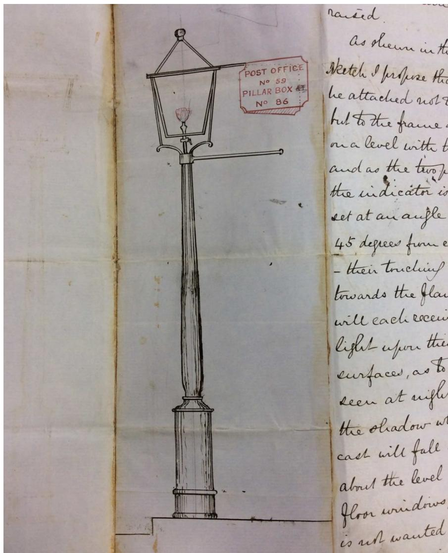
Fig. 152: Design for sign that uses lamppost light to indicate the location of a post office<sup>1275</sup>
