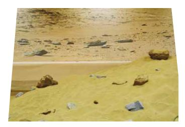
At the Airbus Defence and Space centre in Stevenage, UK, teams of engineers have built a large 'Mars Yard' in order to test the European Space Agency's ExoMars Rover, due to launch in 2018. Unlike other Mars Yards throughout Europe and the USA, this one has been designed specifically to test and perfect the autonomous navigation system ESA will be using to drive their rover across the Martian surface.<sup>1</sup>
