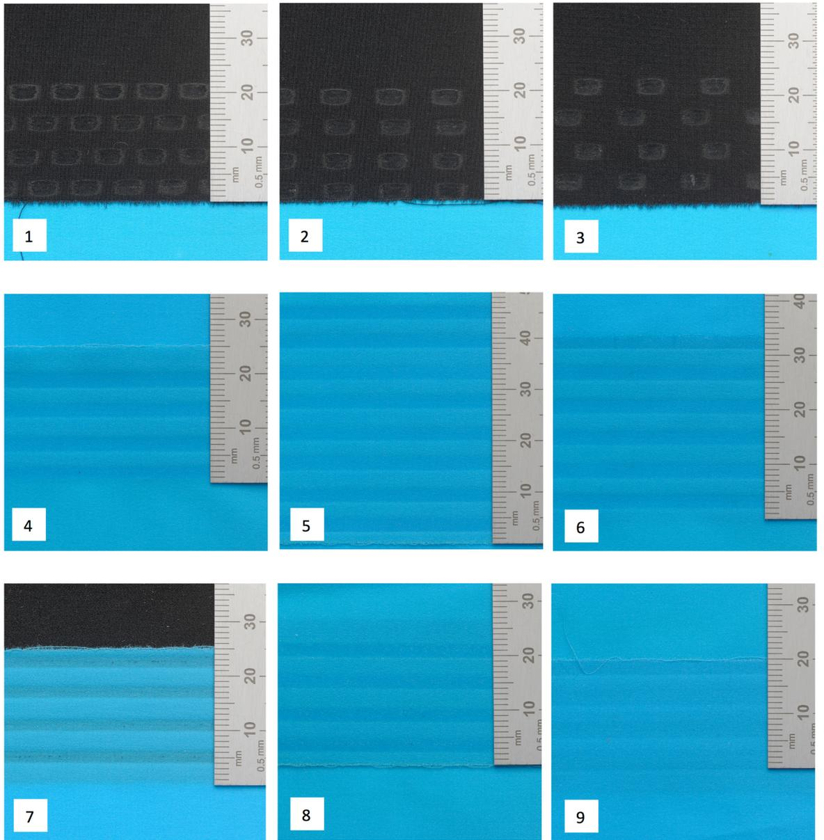
Figure 3.24 9 patterned laser welded seams included in the investigation (Paine 2014)
