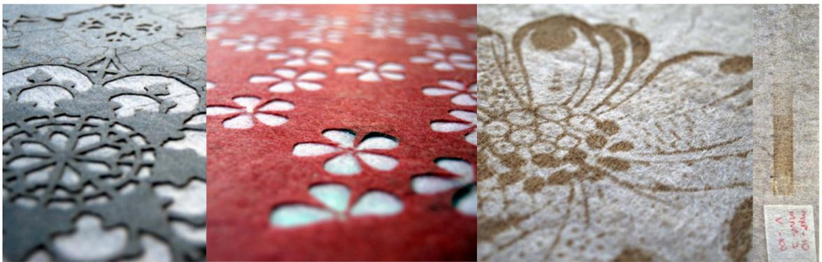
Figure 4.5 Selection of laser-treated non-woven fabrics by Faith Kane(Kane 2009)
