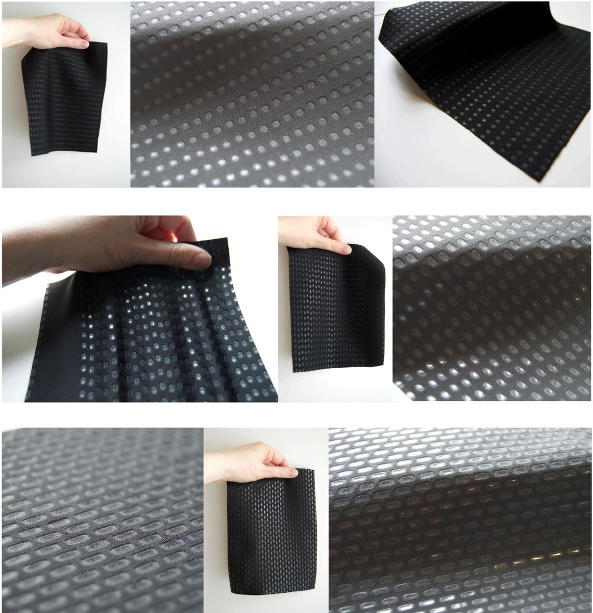
Figure 5.13 (Top) Fabric sample with laser melted spots,  $T_{puls}$  30 ms,  $T_{rep}$  100ms (Paine 2014)
