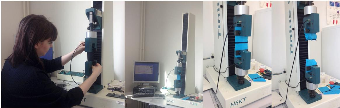
Figure 3.23 Mechanical testing of seams at Speedo (Paine 2014)
