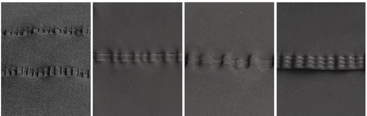
*Figure 3.8 (Left, Centre Left and Centre Right) Examples of ultrasonic seams joined in a lap configuration using continuous ultrasonic welding equipment (Paine 2013)*
