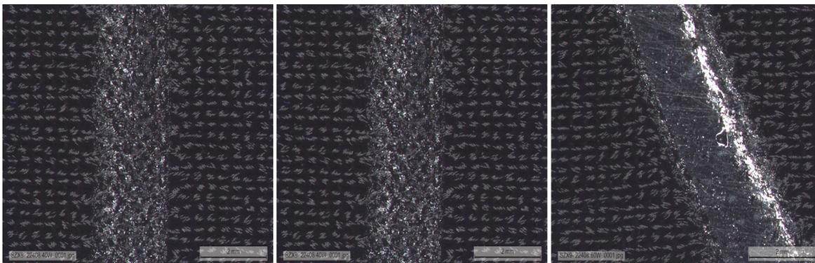
Figure 5.1 (Left) Fabric sample showing laser surface melting created using a power setting of 40W (Paine 2014)
