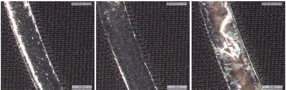
Figure 5.4 (Left) Fabric sample showing laser surface melting created using a speed setting of 3m/min (Paine 2014)
