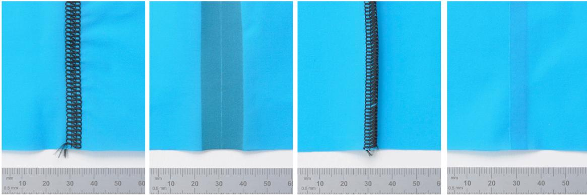
Figure 3.19 (Left) Flat-locked seam (Paine 2014)
