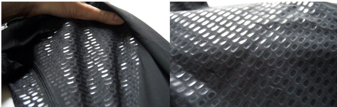
Figure 6.13 Swimsuit prototype with targeted laser-melted panels (Paine 2014)
