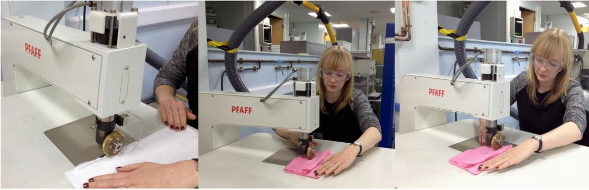
Figure 1.1 Pfaff continuous ultrasonic welding equipment at TWI (TWI 2012)
