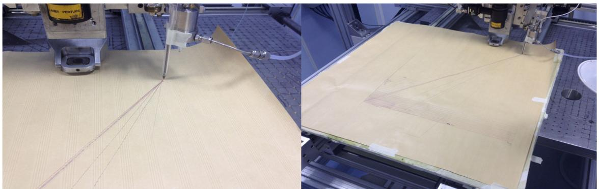
Figure 3.13 Pen attachment to TLW equipment at TWI used to assist in translating the code that moves the x-y table beneath the laser head (Paine 2013)
