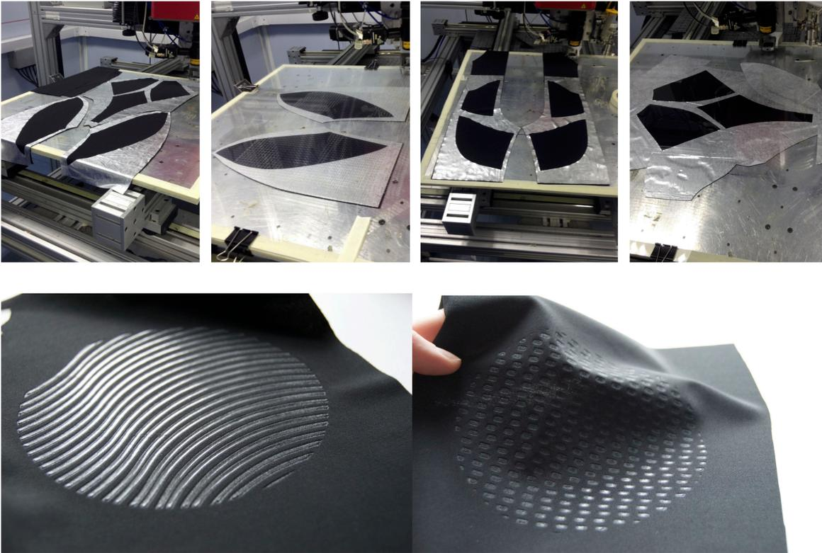
Figure 6.8 (Top) Method of creating targeted zones of compression using reflective stencils and TLW equipment (Paine 2014)
