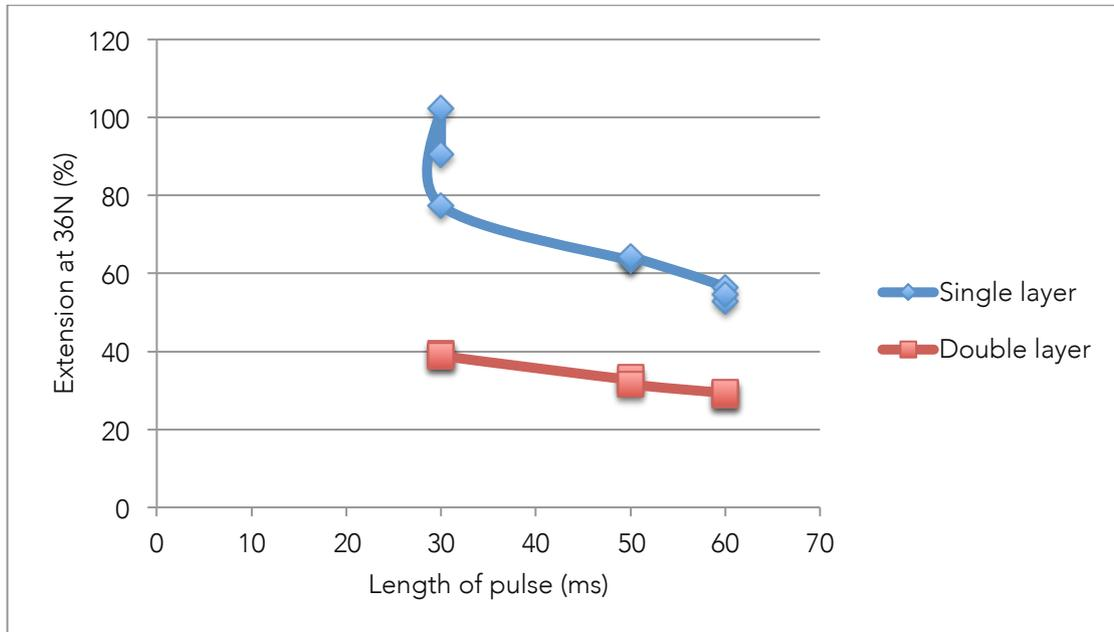
Figure 5.17 Graph showing the effect of pulse density on fabric extension
