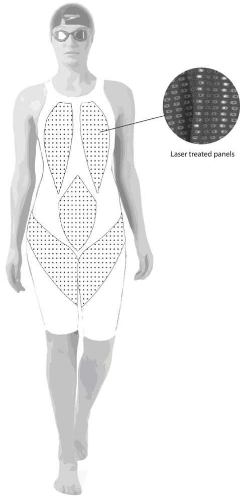
Figure 6.11 Illustration showing placement of panels for swimsuit prototype (author's own)
