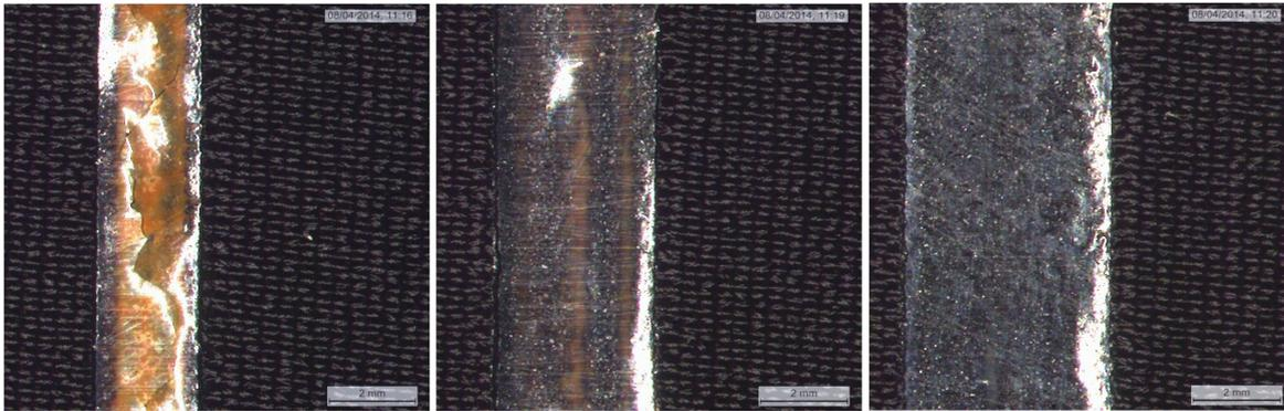
Figure 5.7 (Left) Fabric sample showing laser surface melting created with a laser height of 55mm between x-y table and laser head (Paine 2014)
