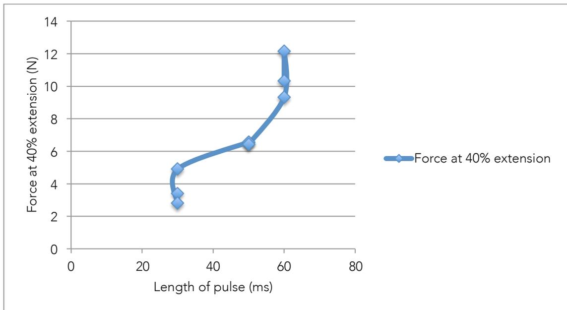
Figure 5.18 Graph showing the effect of pulse density on fabric resistance
