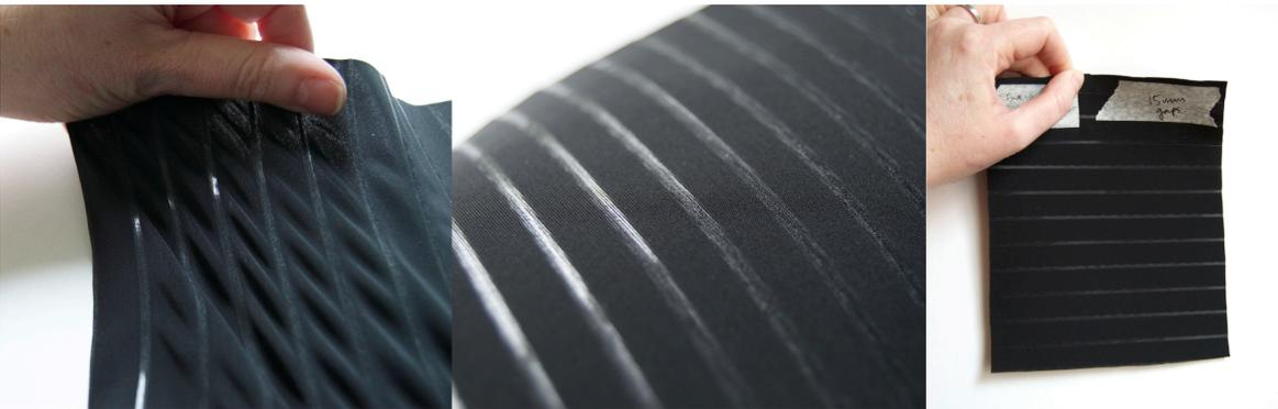
Figure 5.10 (Top) Fabric sample with laser melted lines, 5mm apart (Paine 2014)
