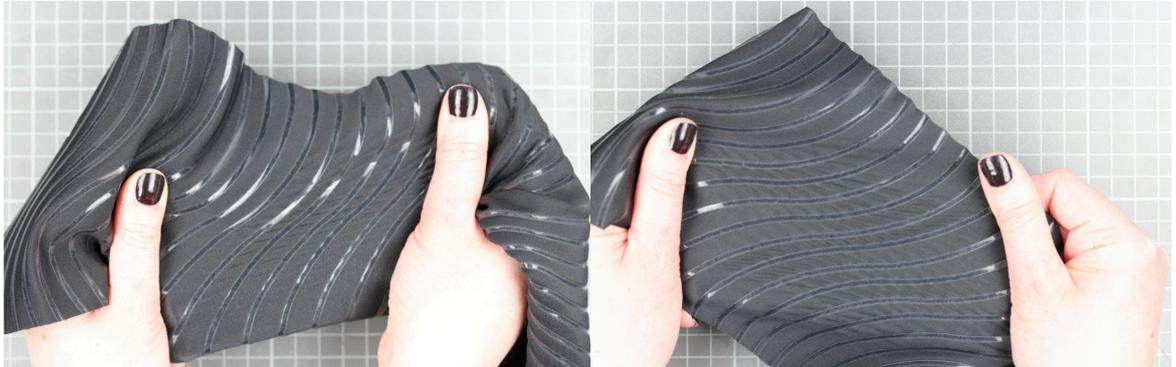
*Figure 3.15 Sample demonstrating the effect of laser surface melting across the full width of a fabric sample (Paine 2013)*
