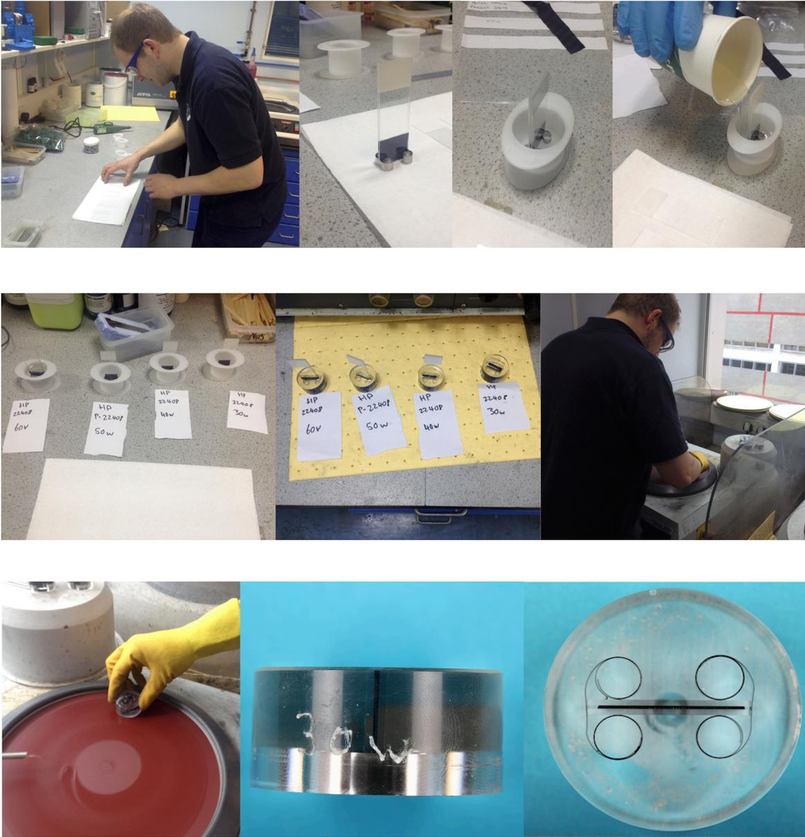
Figure 6.4 Process of mounting and polishing sample for microscopic analysis (Paine 2014)
