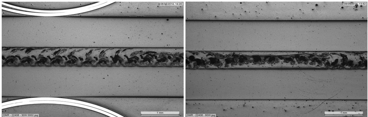
Figure 6.5 (Left) Cross section of fabric sample with surface melting created using a laser power of 30W (TWI 2014)
