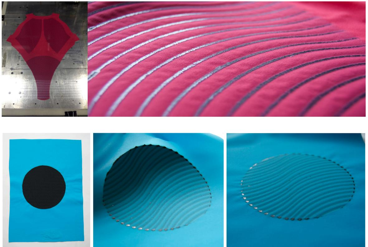
Figure 6.10 Fabric samples with zones of compression created using absorptive lower panels and TLW equipment (Paine 2014)
