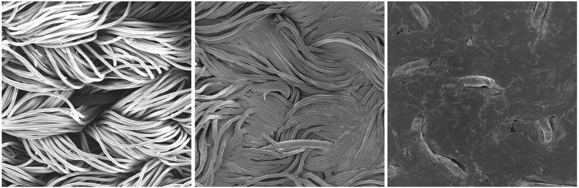
Figure 3.1 (Left) SEM image of an unwelded sample of stretchy jersey fabric (TWI 2012)
