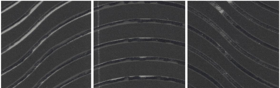
Figure 6.1 (Left) Fabric sample showing left side of curved laser melted pattern (Paine 2014)
