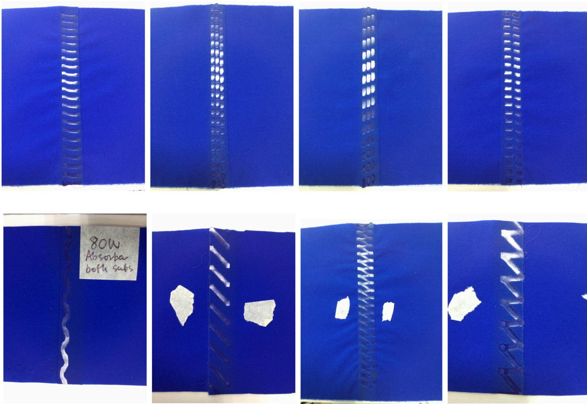
Figure 3.14 Fabric samples showing a variety of decorative patterned laser welded seams (Paine 2013)
