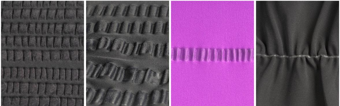
Figure 3.11 (Left, Centre Left, Centre Right) Fabric samples demonstrating all-over rippled surface effect created using ultrasonic welding equipment (Paine 2013)
