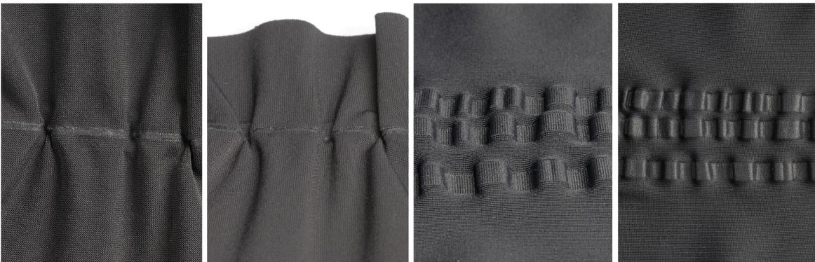
*Figure 3.16 (Centre Right, Right,) Fabric samples demonstrating ruched effect created using polyurethane tape and laser welding equipment (Paine 2013)*
