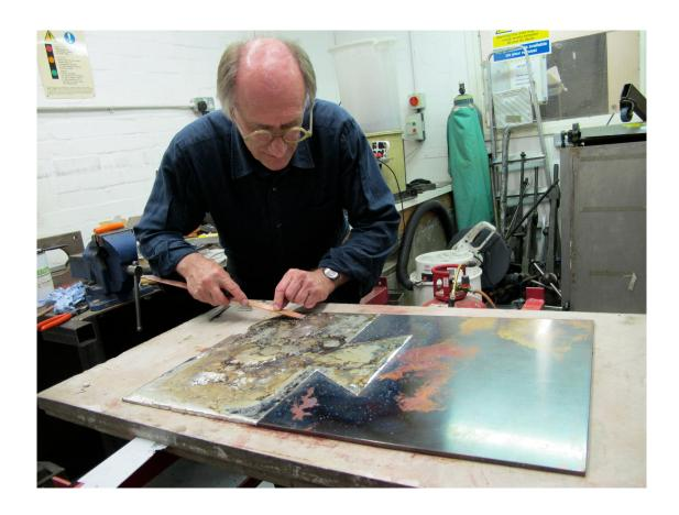
11. Cleaning up the surface of tin melted onto a copper plate.
