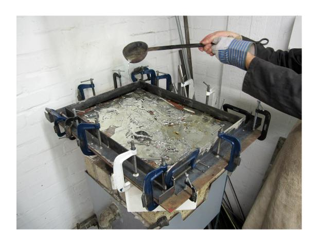
10. Set-up for casting tin onto a copper plate.
