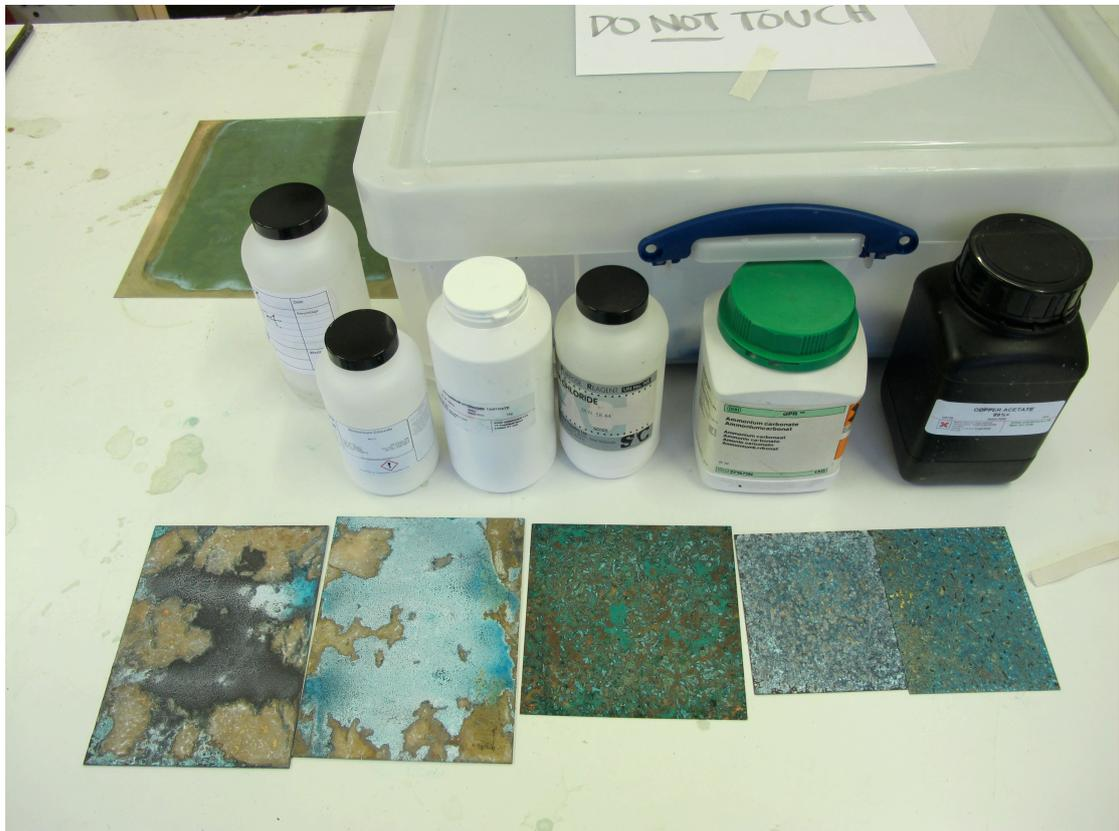
9. Samples of patinated copper and brass plates using the sawdust and cotton wool techniques.
