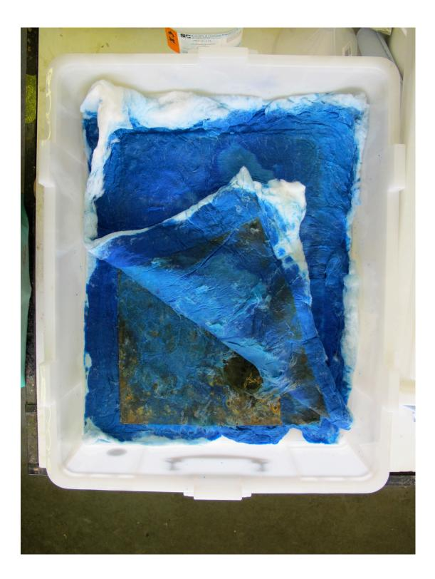
8. Set-up for patinating the copper and brass plates using the cotton wool process.
