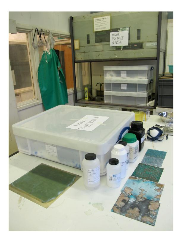
7. Chemical laboratory set-up for patinating the copper and brass plates.
