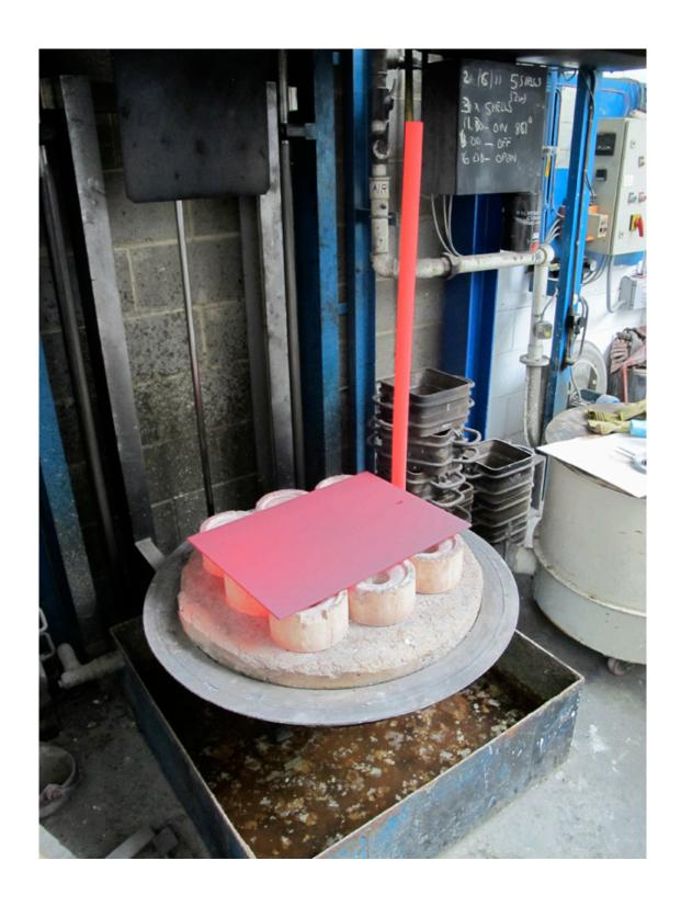
4. Soaking the copper plates at red-heat.
