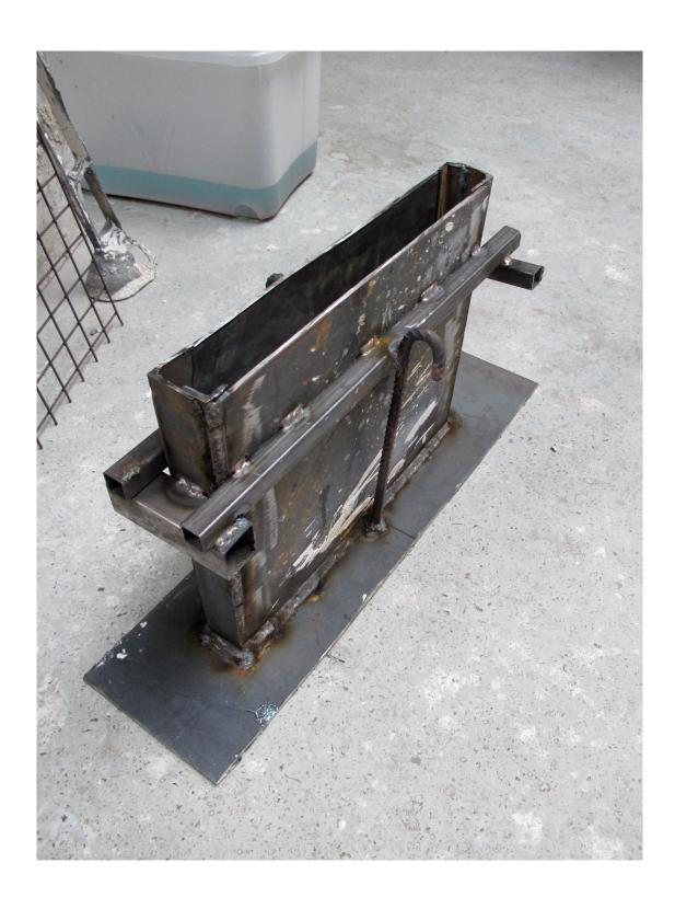
3. Purpose-built tank for dip-tinning the copper plate.
