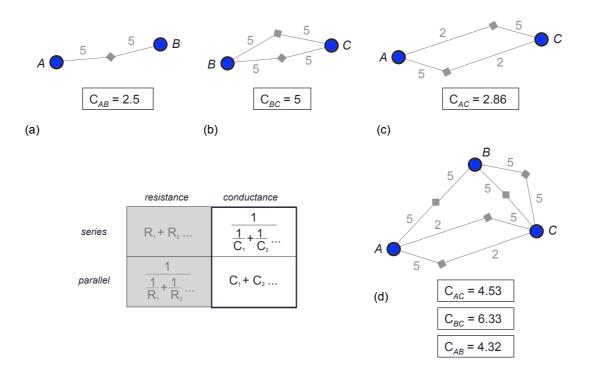
actors) would contribute to a lesser extent owing to their greater length. Example conductance calculations and values for simple networks are illustrated in Figure E-7.
