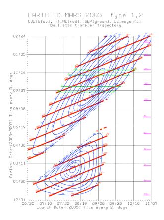
Figure 7-2 Example Porkchop Plot for 2005 This plot shows launch "windows", arrival dates and accessible latitudes for ballistic trajectories. It is representative of, but is not the actual chart used by the team in this study. Source: JPL "Porkchop' is the First Menu Item on a Trip to Mars." <http://mars.jpl.nasa.gov/spotlight/porkchopAll.html>
