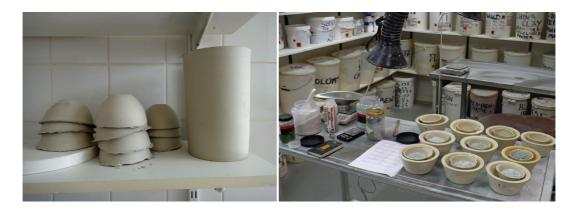
Slip cast and bisque fired crucibles (left). Mixing batch with oxides. The crucibles are placed in trays for firing (right).
