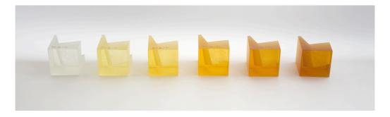
$3 \text{ cm}^3$  cubes coloured with cerium oxide and titanium dioxide in the ratio 1:1. From left: 1%, 2%, 3%, 4%, 5%, and 6% of each oxide.
