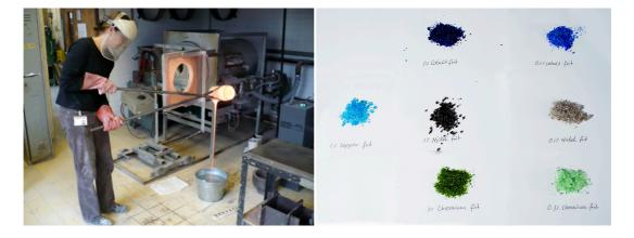
Figure 48: Hot glass is poured into water to produce frit.
