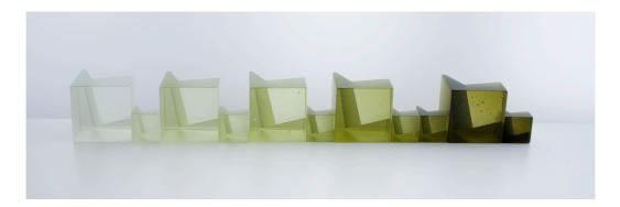
Figure 75: 3 cm<sup>3</sup> and 6 cm<sup>3</sup> cubes coloured with red iron oxide. From left: 0.1% (6cm<sup>3</sup> only), 0.3%, 0.5%, 1%, 1.5% (3 cm<sup>3</sup> only), 2% and 3% (3 cm<sup>3</sup> only).
