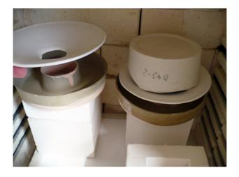
Figure 62: The broken crucible is suspended upside-down over the mould using custom-made ceramic props.
