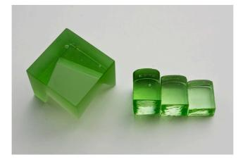
Figure 112: glass coloured with 0.01% chromium oxide. Cube: 6 cm<sup>3</sup>. Thickness of bars: 4 cm, 3 cm and 2 cm.
