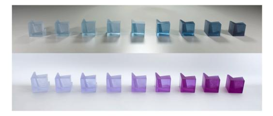
$3 \text{ cm}^3$  cubes coloured with neodymium oxide, in fluorescent light (top) and incandescent light. From left: 0.25%, 0.5%, 1%, 2%, 3%, 4%, 8%, 10% and 15%.
