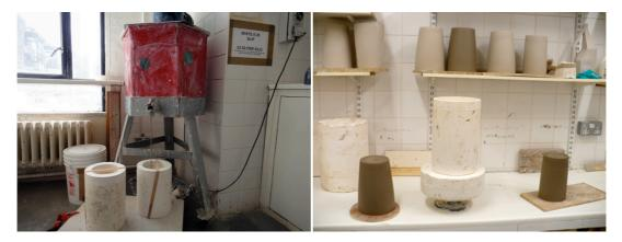
Figure 57: Slip-casting of crucibles.
