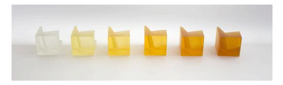
Figure 77: 3 cm<sup>3</sup> cubes coloured with cerium oxide and titanium dioxide in the ratio 1:1. From left: 1%, 2%, 3%, 4%, 5%, and 6% of each oxide.
