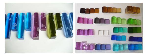
Figure 64: Test bars hot-cast into graphite moulds (left) and cut and polished for spectrophotometer measurements (right). W: 2.5 cm.
