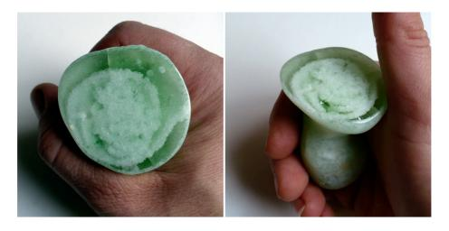
Figure 45: Devitrification in RG2 Glass coloured with 0.01% chromium oxide. Diameter: 4.5 cm, L: 6.5 cm.
