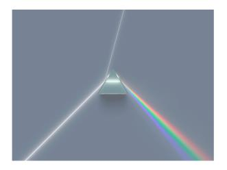
Figure 31: Light dispersion in a triangular prism
