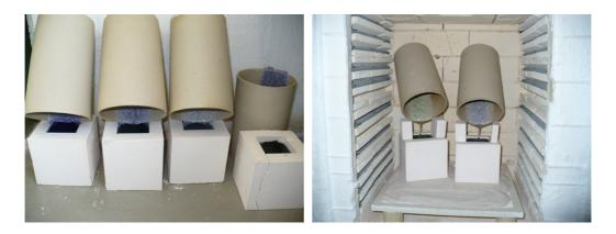
Figure 61: The crucibles adhere to the cast, causing the glass to crack (left). The crucible is suspended above the mould (right).
