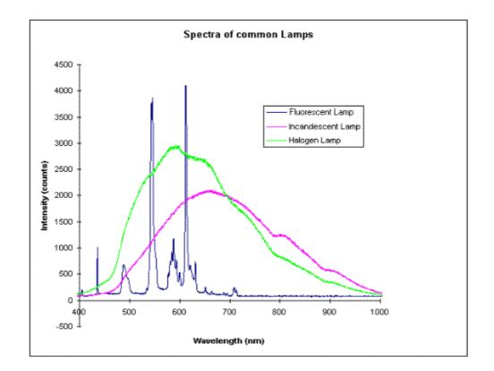
Figure 42: Spectra of common lamps. (<u>http://www1.union.edu/newmanj/lasers/Light%20Production/LampSpectra</u>.gif, accessed 09/05/09)
