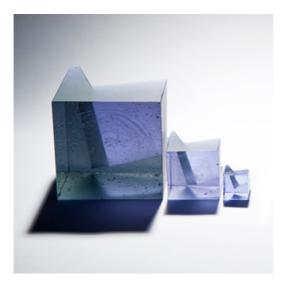
Figure 69: scaling up and down. Glass coloured with 2% neodymium and 0.005% chromium oxide. 12 cm<sup>3</sup>, 6 cm<sup>3</sup>, 3 cm<sup>3</sup>. Photograph: Ester Segarra.
