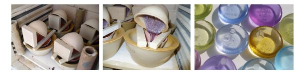
Figure 53: initial set-up for casting small hue tests. Diameter: 5 cm.
