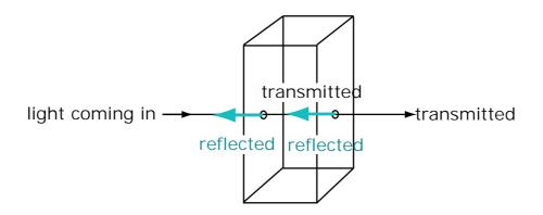
Figure 29: Reflection and transmission
