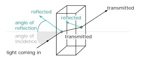
angle of incidence = angle of reflection
