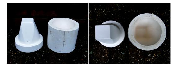
Plug for taking plaster mould off and resulting plaster mould for slip-casting clay kiln casting moulds for basic tests.
