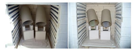
Crucible kiln casting. Before (left) and after the firing (right).
