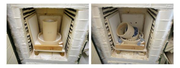
Figure 59: Earthstone handbuilding white ES20 crucible with Glasma frit before (left) and after firing.
