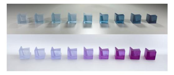
Figure 76: 3 cm<sup>3</sup> cubes coloured with neodymium oxide, in fluorescent light (top) and incandescent light. From left: 0.25%, 0.5%, 1%, 2%, 3%, 4%, 8%, 10& and 15%.
