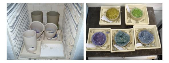
Figure 58: Porcelain crucibles (left) and HT Stoneware crucibles after firing.
