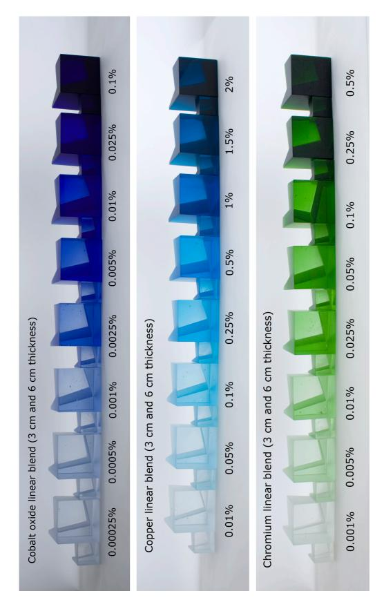
Plate 19: Cobalt, copper and chromium oxide linear blends.
