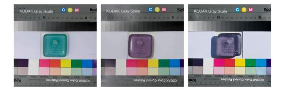
Figure 56: Sample no. 29-10 (3% neodymium oxide, 0.0075% chromium oxide) in fluorescent light, incandescent light and daylight. W: 5 cm.
