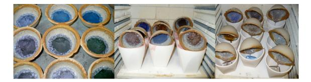
Figure 54: Improved set-up for casting small hue tests.
