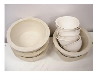
Figure 50: Initial stoneware crucibles, later to be used as trays to guard against spillage, and small porcelain crucibles.
