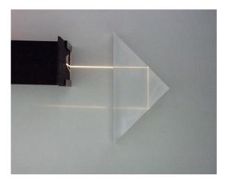
Figure 32: Reflection of light in a Porro Prism
