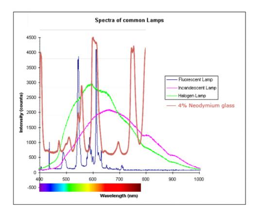
Figure 44: Interaction between absorption spectrum of 4% neodymium glass and emission spectrum of fluorescent, incandescent and halogen lamps.
