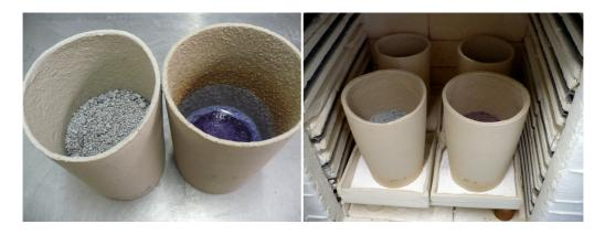
Tall crucible with glass batch, and with glass after firing (left). Crucibles with batch are set up in a kiln on trays with calcined alumina, ready for firing (right).
