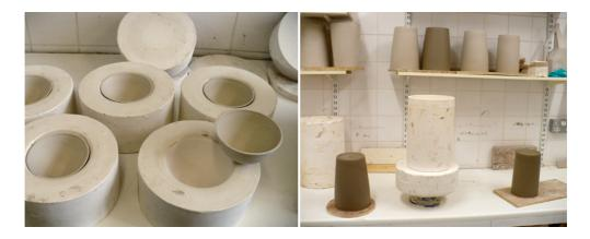
Slip-casting moulds with crucibles.
