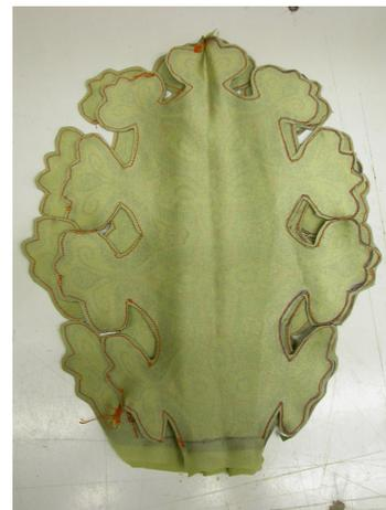
Heat pressing the panels together accurately using plastisol ink as a glue
