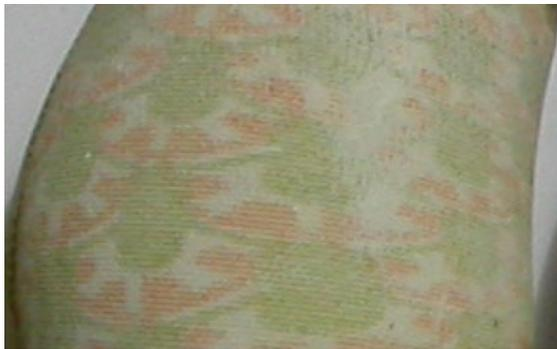
Fully stretched and fired. Illustrating the issues of reducing saturation of ink
