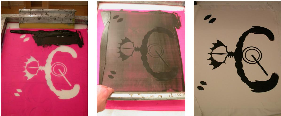
Fig 11. Drawing the squeegee across the screen pushes the ink through the open areas of mesh (defined by the stencil mask) and leaves a deposit on the surface of the substrate beneath
