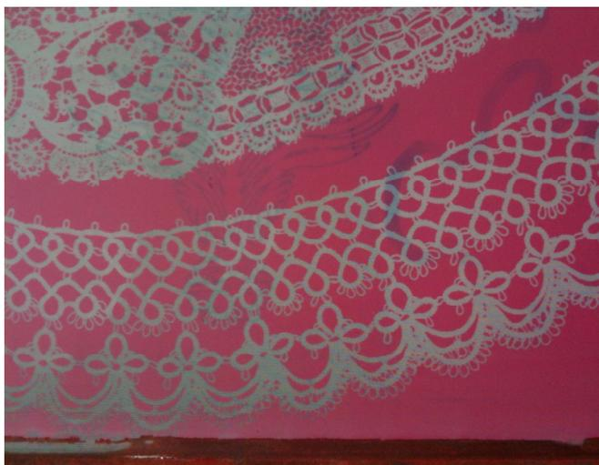
Fig 36. Photo-stencil produced using lace to physically block the light from hardening the photo-emulsion
