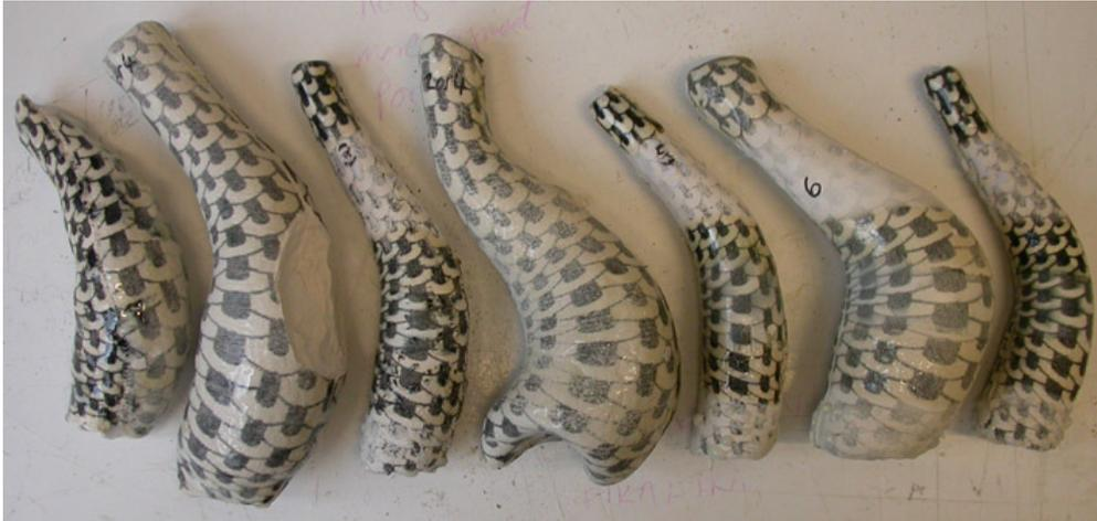
Low temperature frit tests, aiming to seal the print onto the clay surface
