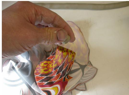
For medium sized cavities I dropped small clay balls into the mould and used a tool to compact them
