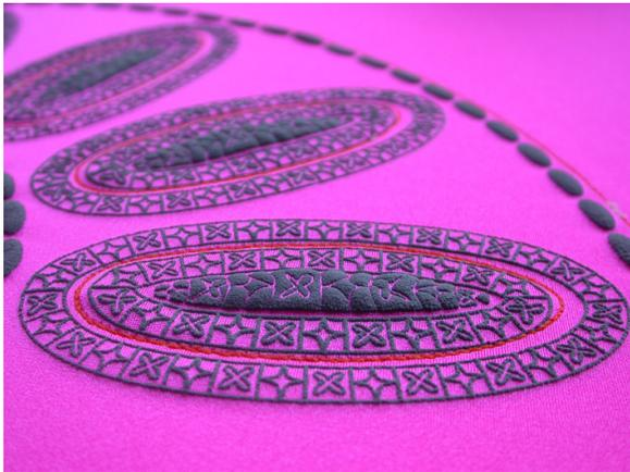
Expanding base loaded with ceramic pigment
