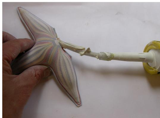
For small elements I mixed a thick paste and injected this into the mould with a caulk gun
