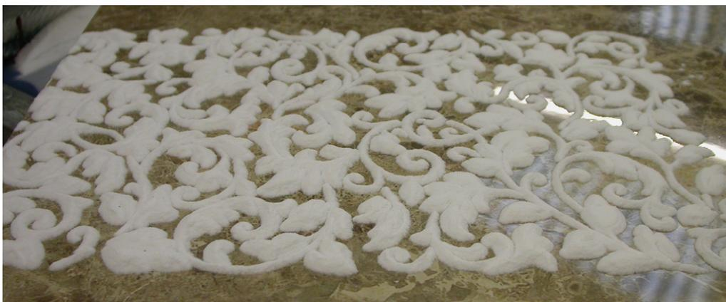
Fig 25. Vitrosa frit powder deposit before being fired
