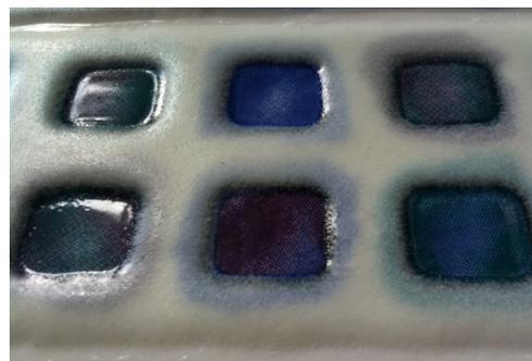
Fig 26. Various samples of 'Vitrosa' tile work at Johnson Tiles Ltd. The effects range from (top right) selectively and partially obscuring the underlying image – (bottom right) selectively and partially obscuring whilst adding dimension – (bottom left) adding translucent gloss dimension over an image – (top left) adding opaque relief to fit within a print
