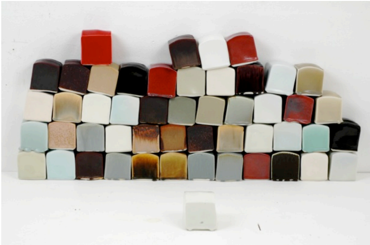
Raw glazing vs. application over biscuit
