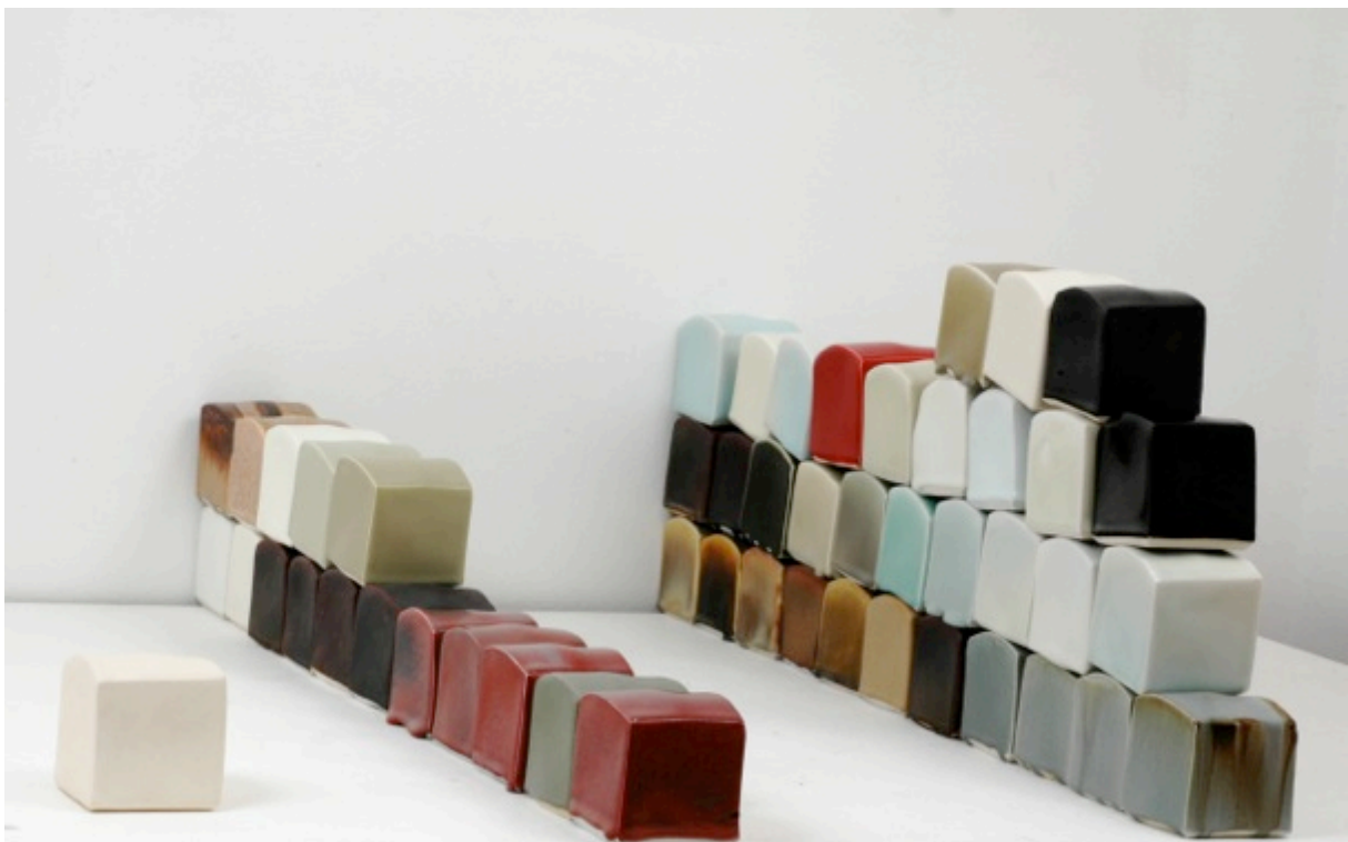
Classification of Cobblestones according to relative fusibility
