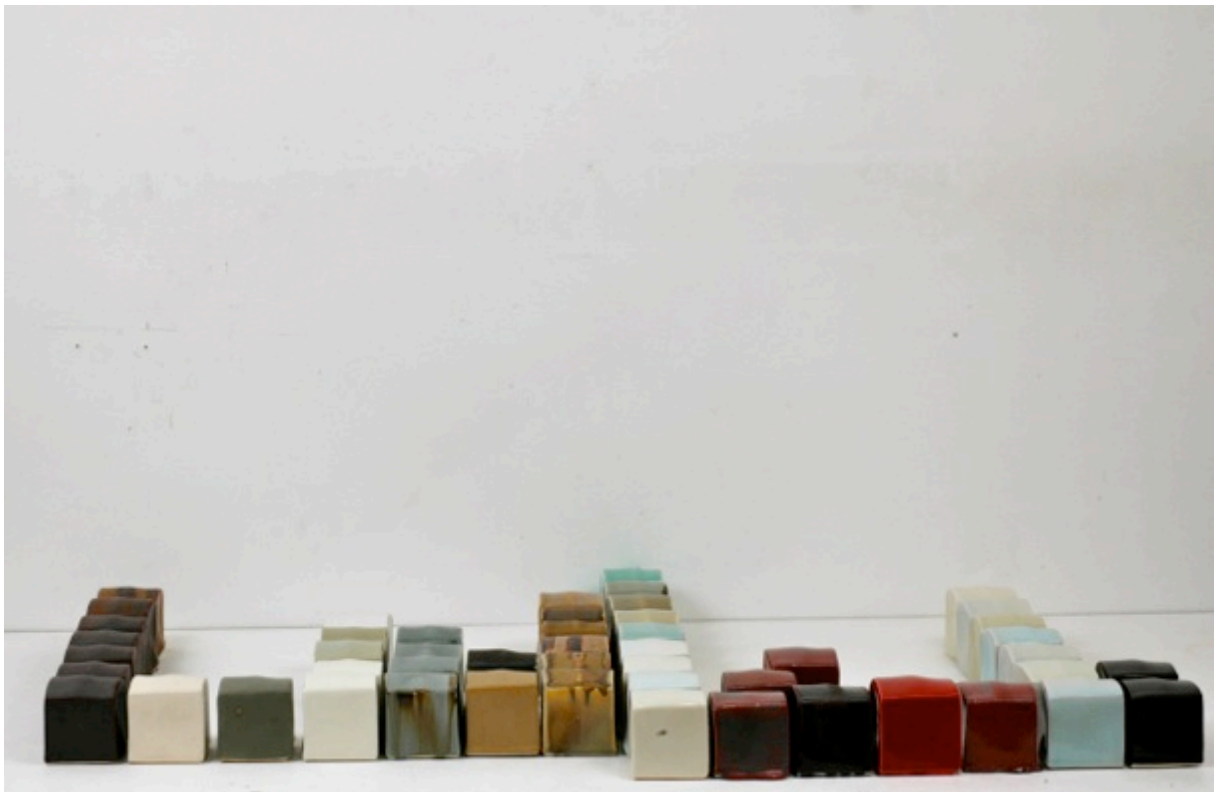
Classification of Cobblestones according to mattness
