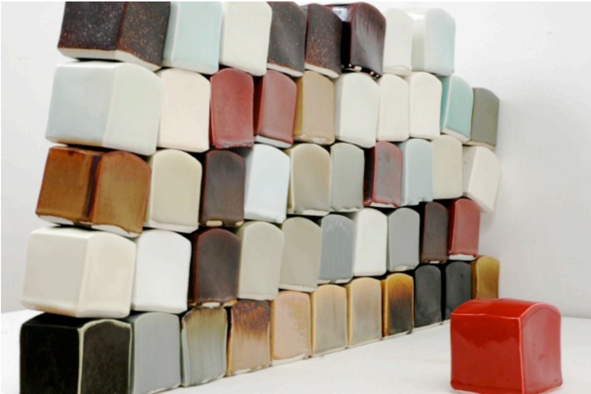
High temperature glazes (stoneware and porcelain) vs. low temperature glazes (earthenware)
